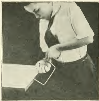
Fig. 23. Removing the saw-blade
