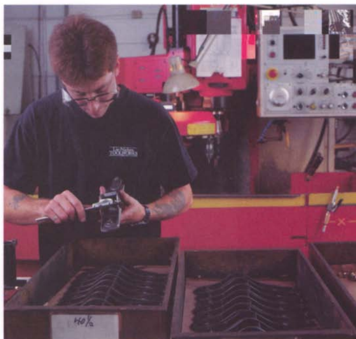
As each rough casting passes through the machine shop getting its body milled to size, its sole ground flat, and its throat opened, operators constantly check tolerances and quality.
