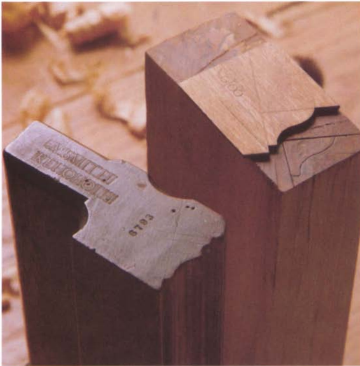
The molding profile is scribed on the toe and heel from a wooden template. For some profiles, the molding is “sprung” or angled for a more consistent throat, as can be seen on the old molding plane on the left.
