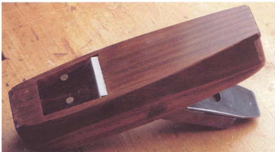
The new throat piece on this lignum-vitae smoother is secured in place with glue and screws.
