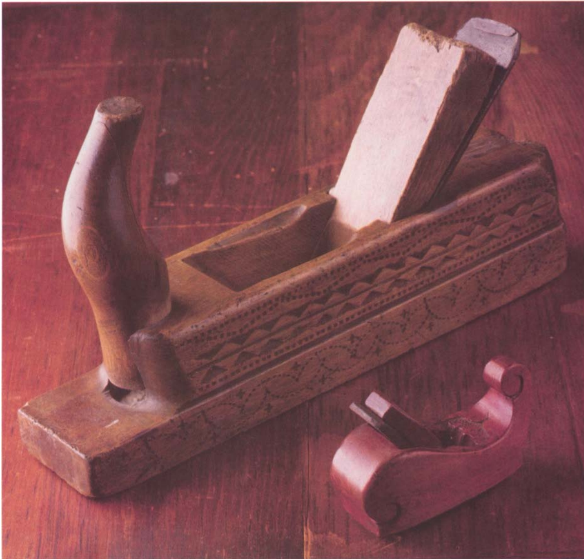
These two horn planes show the upright handle and decorative detailing characteristic of European planes.
