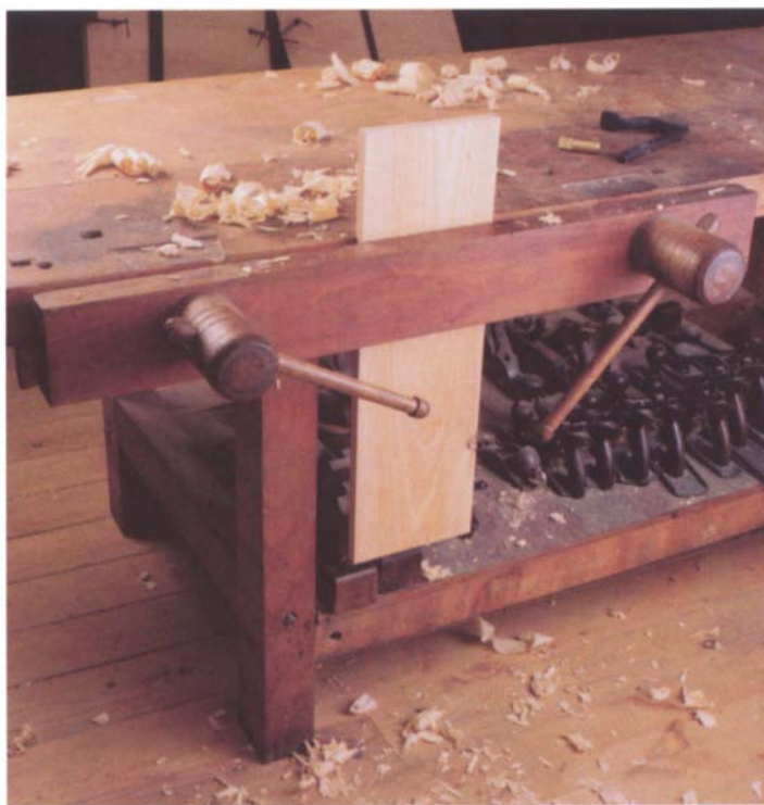
A side vise with two large wooden screws is ideal for clamping wide boards upright for planing end grain.
