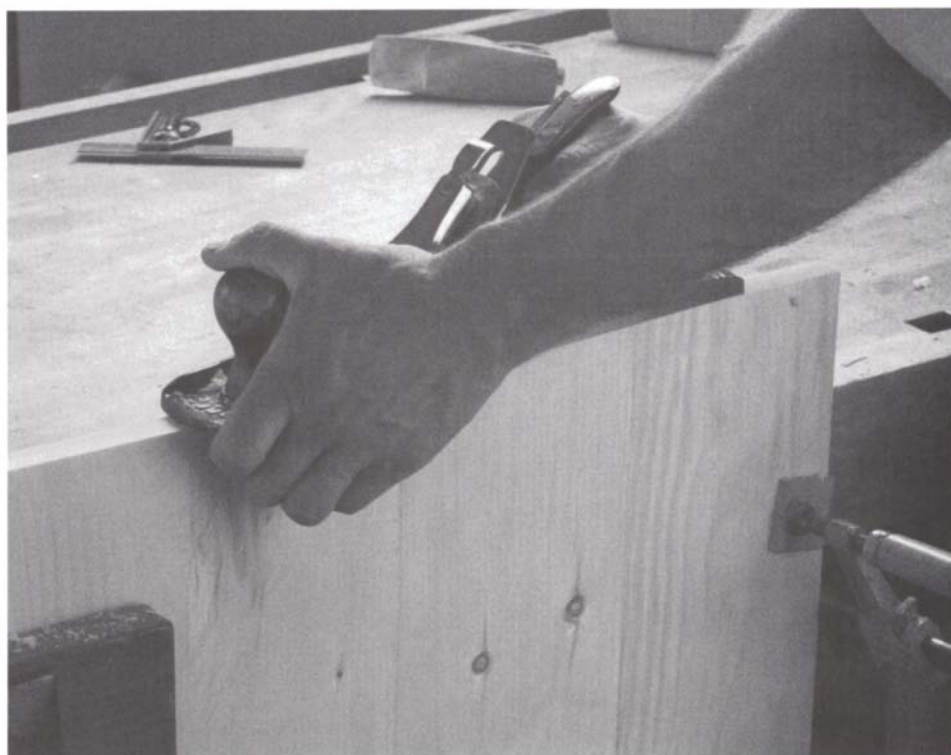
Shooting a long end-grain edge with a #5 or longer bench plane works well. A #5 cuts a true edge and is easier to hold and use than a smaller block plane.
