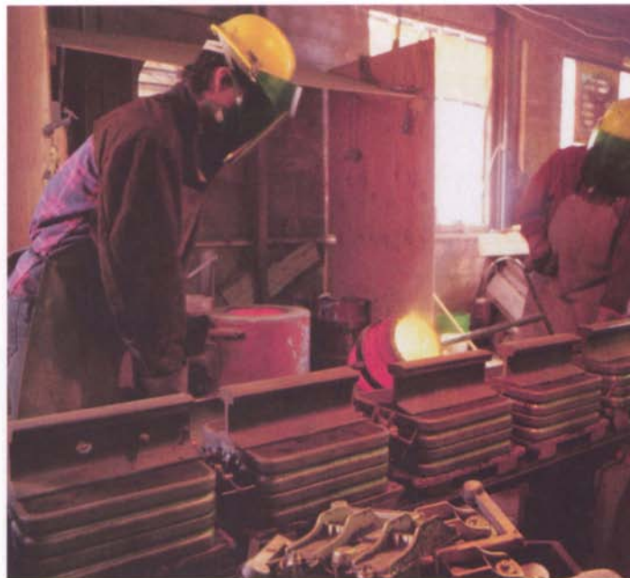
Plane bodies and other parts are cast in small batches in traditional sand molds. The heavy bars atop the molds prevent the sand from buckling as the molten metal fills the mold.
