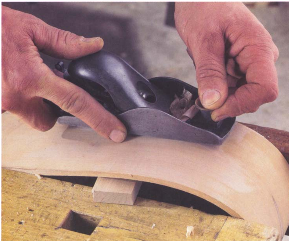
A block plane works well for smoothing convex surfaces. The trick is to rock the plane, keeping it tangential to the surface and firmly engaged so that it cuts continuously without chattering.
