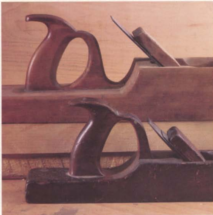
Razee handles lower the plane's center of gravity and deliver the force of your hand right to the cutting action of the plane.
