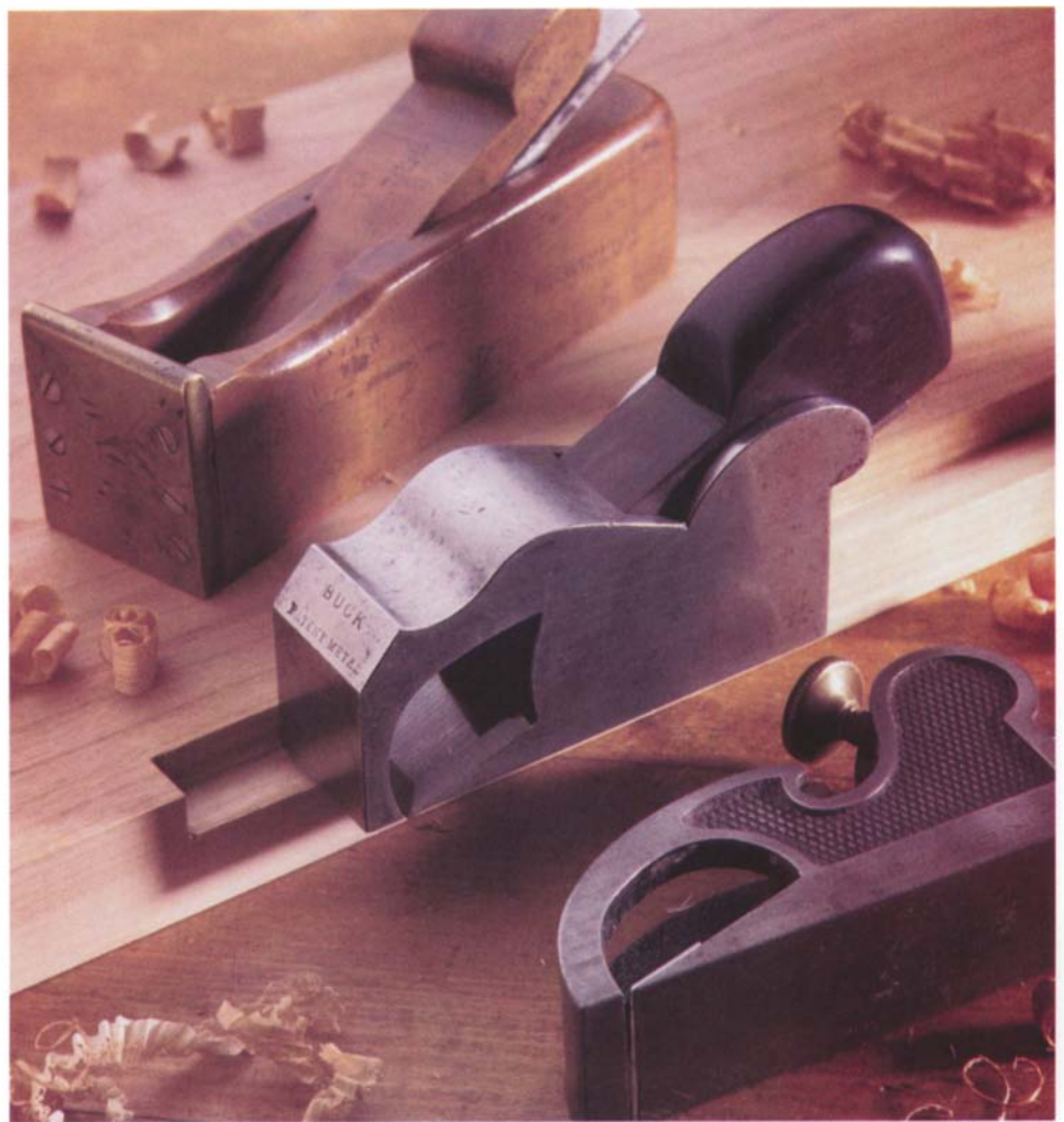
The best planes for cutting stopped rabbets are of a bullnose design, with the iron set close to the toe. At rear is a craftsman-made boxwood and brass bullnose plane; in the center, a shapely English bullnose with ebony wedge; and at bottom an E. Preston English bullnose similar to a Stanley design.
