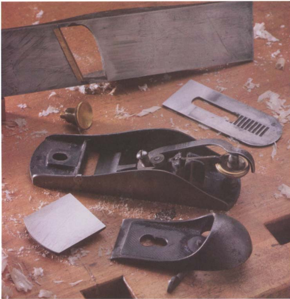
A block plane disassembled shows its single iron, adjuster, cam-locking lever cap, adjustable toe piece and the knob that secures it, and low bed angle. Too low a bed angle is fragile, as shown by the skewed block plane in the background whose bed has cracked away.
