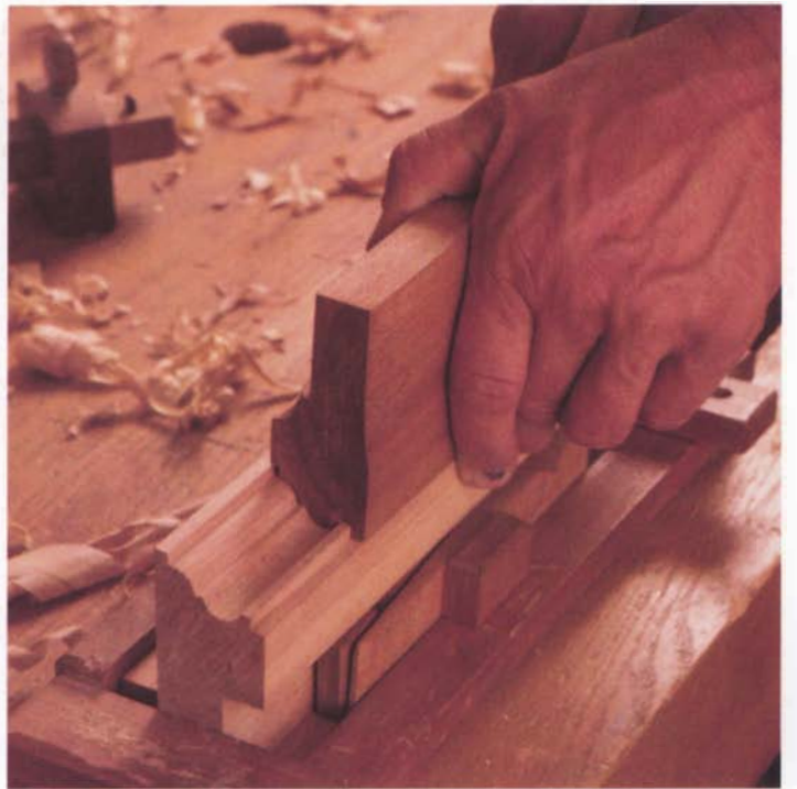
Commercial plane makers shape the sole with a “mother” or backing plane with a mirror-image sole profile.
