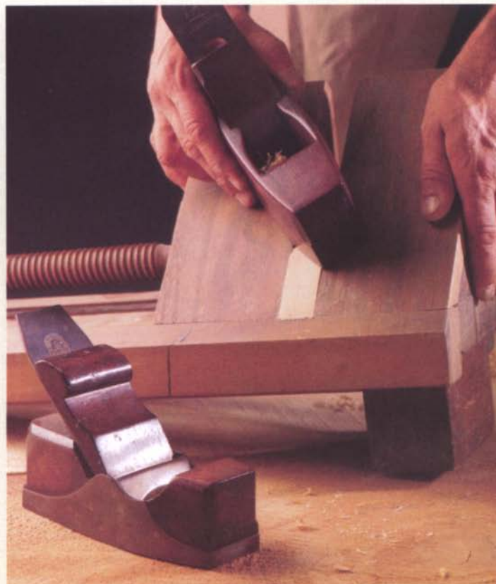
A miter shooting clamp guides a plane to cut accurate miters on any work that can be clamped between the jaws.
