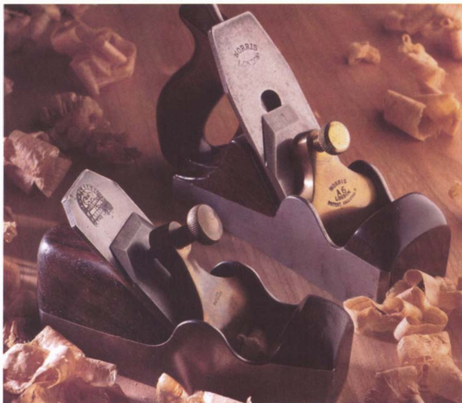
Some of the most beautiful and effective smoothing planes ever produced were made in Britain up until early in this century. Both the A6 Norris (rear) and #6 Spiers are massive, with thick irons and tight throats.
