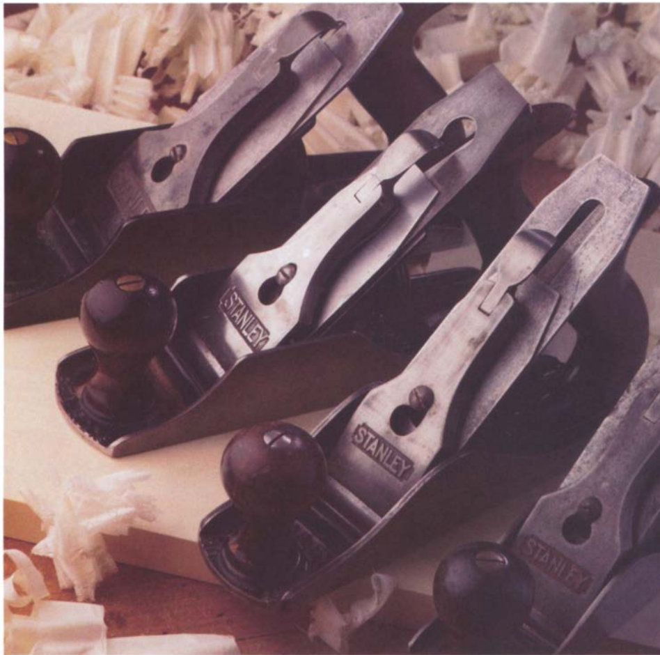
Bailey-pattern smoothing planes include the #2 and #3 (foreground). The Bed Rocks #604 and #604½ at rear are ideal for smoothing all but the most highly figured woods.
