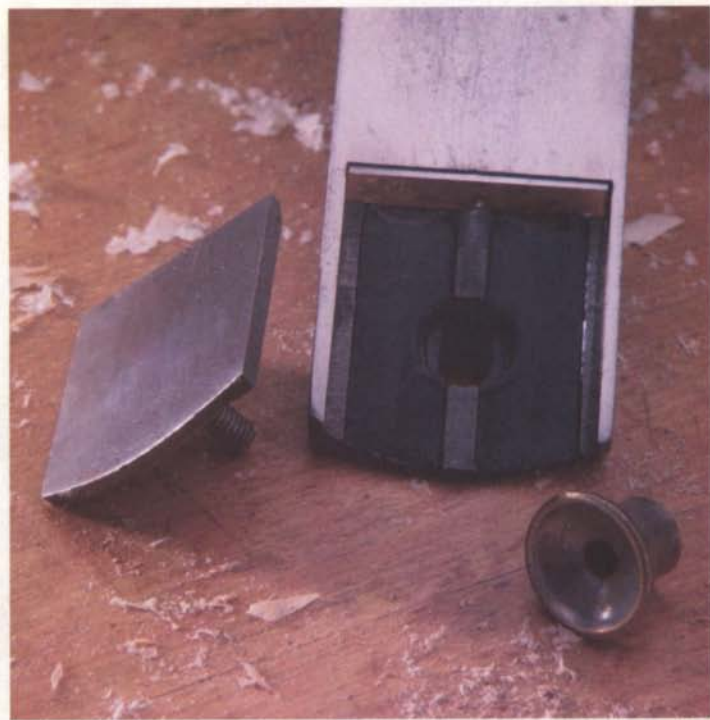
The adjustable toe piece is secured to the plane body with a knurled knob.
