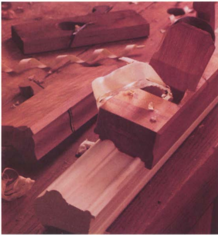
A large handrail plane (at right) shapes the sides of straight or gently curving sections of handrail. An ogee, hollow, or capping plane (at left) cuts the rounded top profile.
