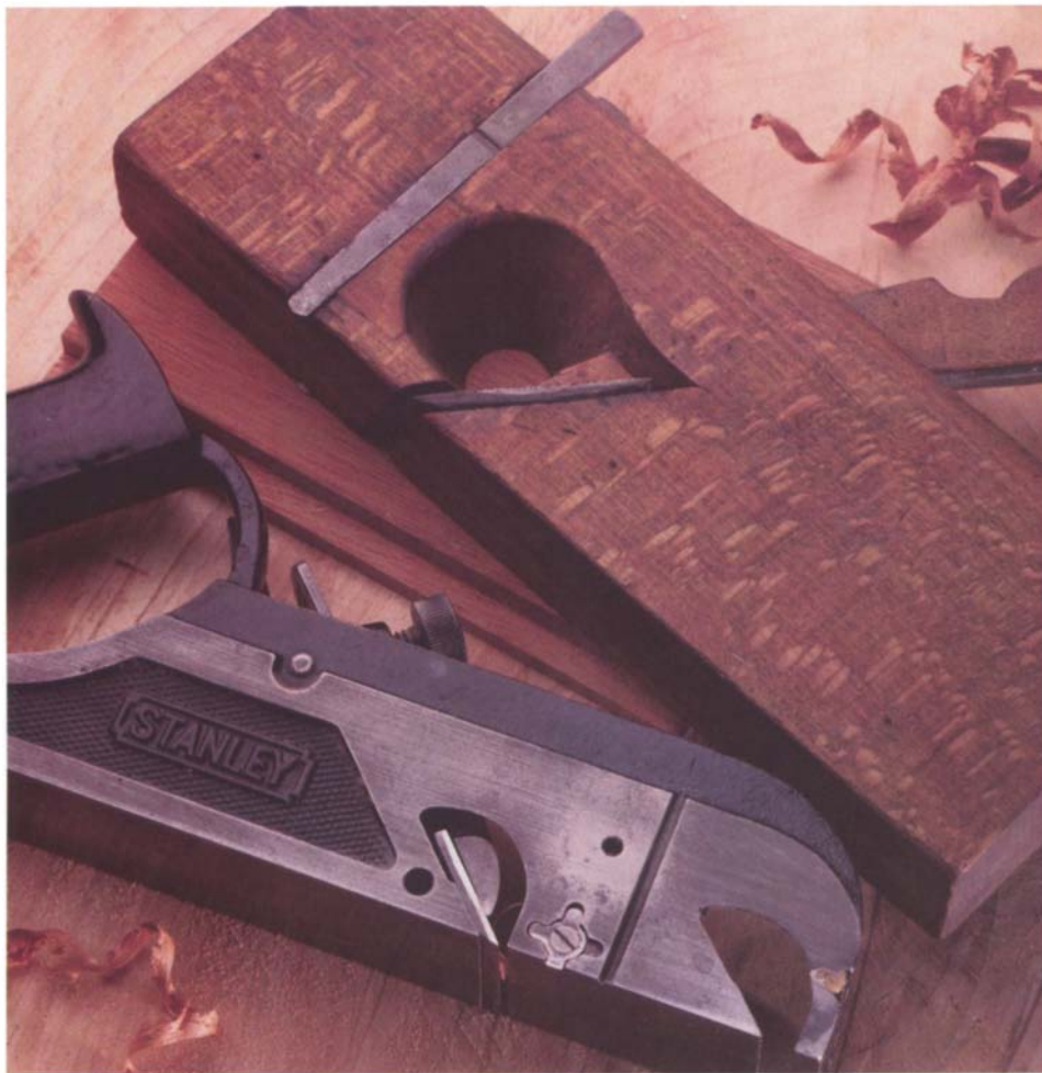
Nickers score the fibers on cross grain ahead of the iron for a clean sharp rabbet. Shown here are a Stanley “wheel” type nicker with individual spurs and a wooden rabbet with a knife-like nicker dovetailed into the side of the plane. The notch filed into the side of the nicker is used to adjust its depth.
