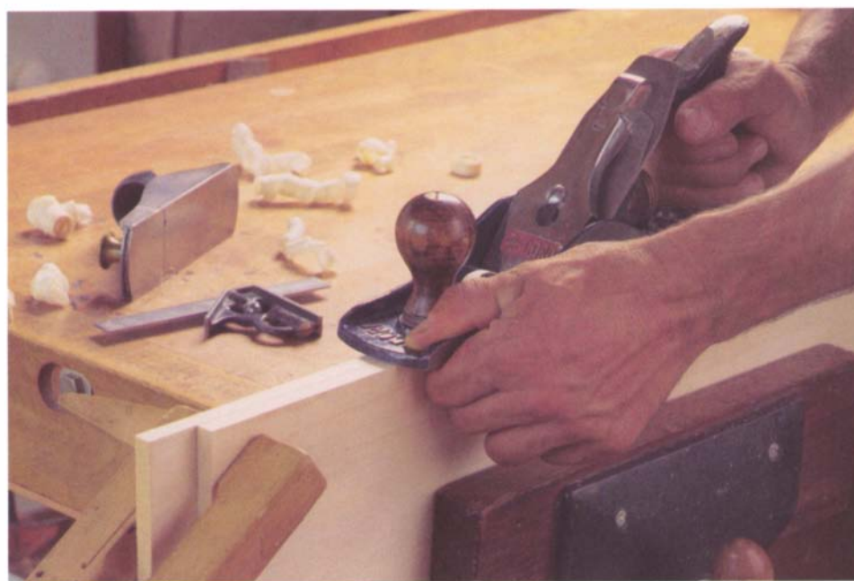
To joint boards in pairs, fold the boards together, line up the edges to be jointed, and clamp securely.
