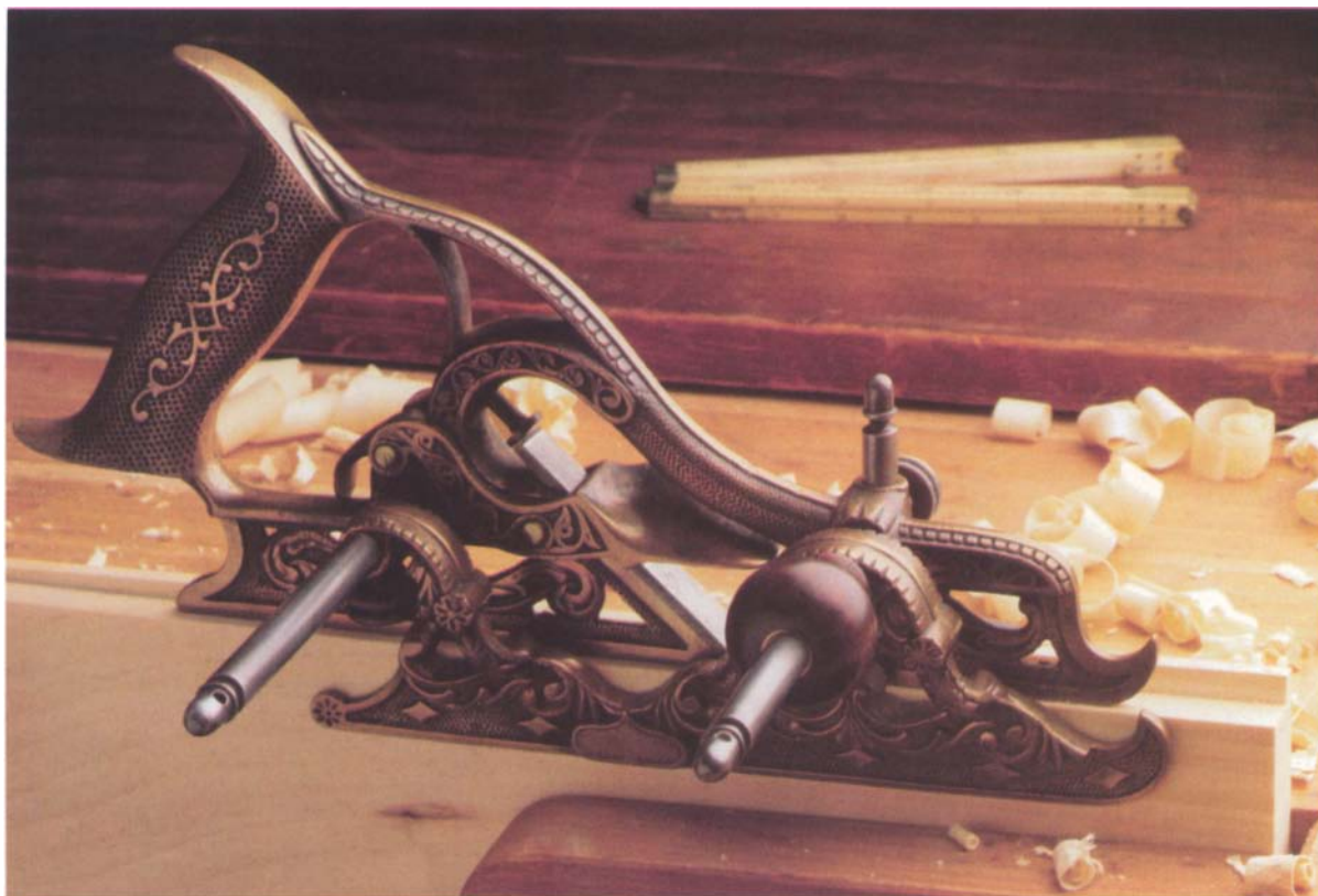
The closed "D" handle of this rare Miller's Improved Joiner's plow plane, in gunmetal with beautiful floral decoration, is formed as part of the casting.
