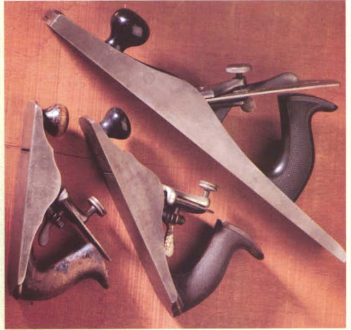
Many innovative approaches were tried for adjusting the irons of cast-iron planes. On Chaplin's improved patent bench planes a large nickel-plated lever moves the "saddle" that holds the iron in or out.
