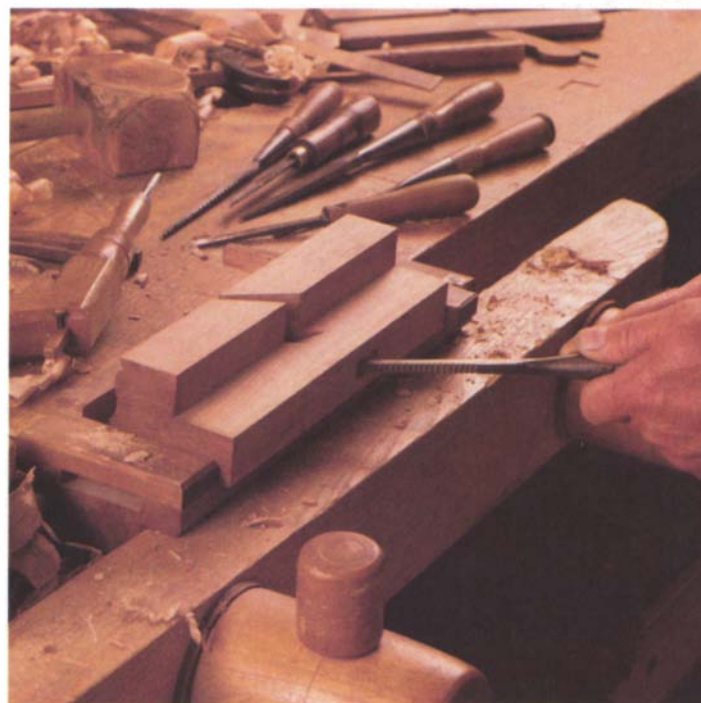
The mouth and throat of the plane are cut with a fine backsaw and then chopped out with a chisel. The pitchboard in the background is for laying out the throat opening.
