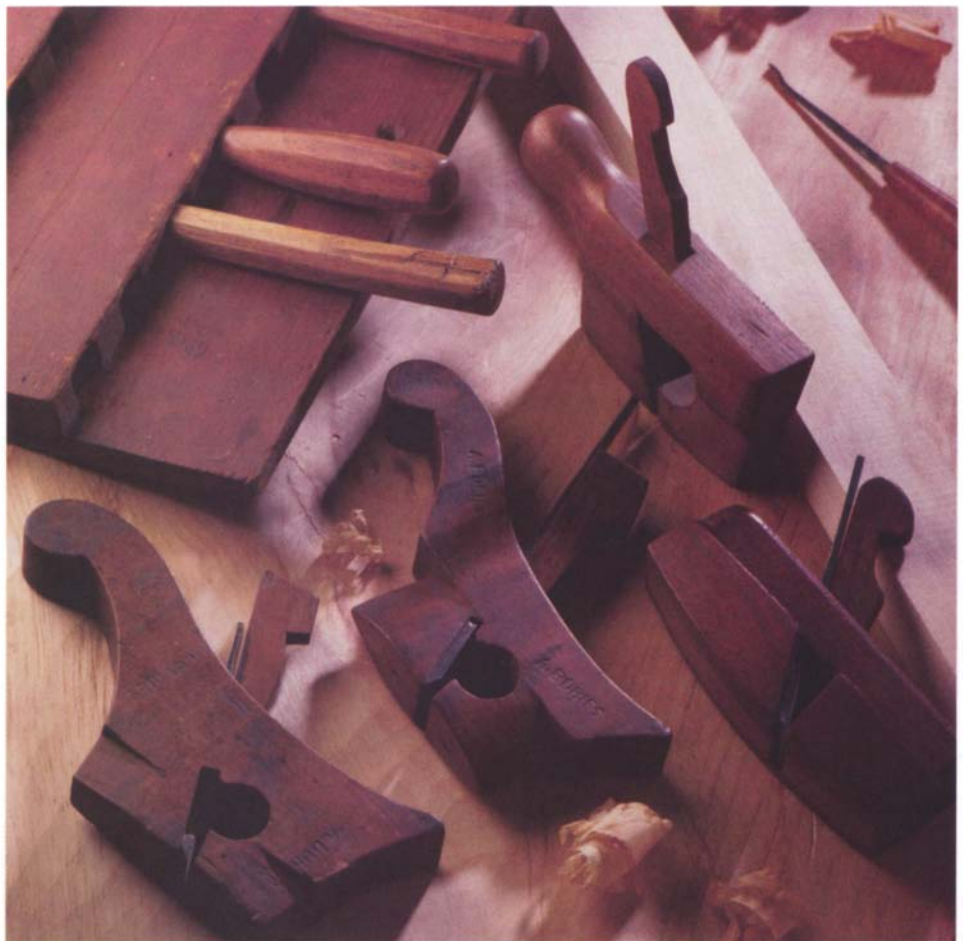
A coachmaker needed short-soled planes to work curved parts. The shape of the plane body evolved to an elegant and functional pistol grip, allowing one-handed control.
