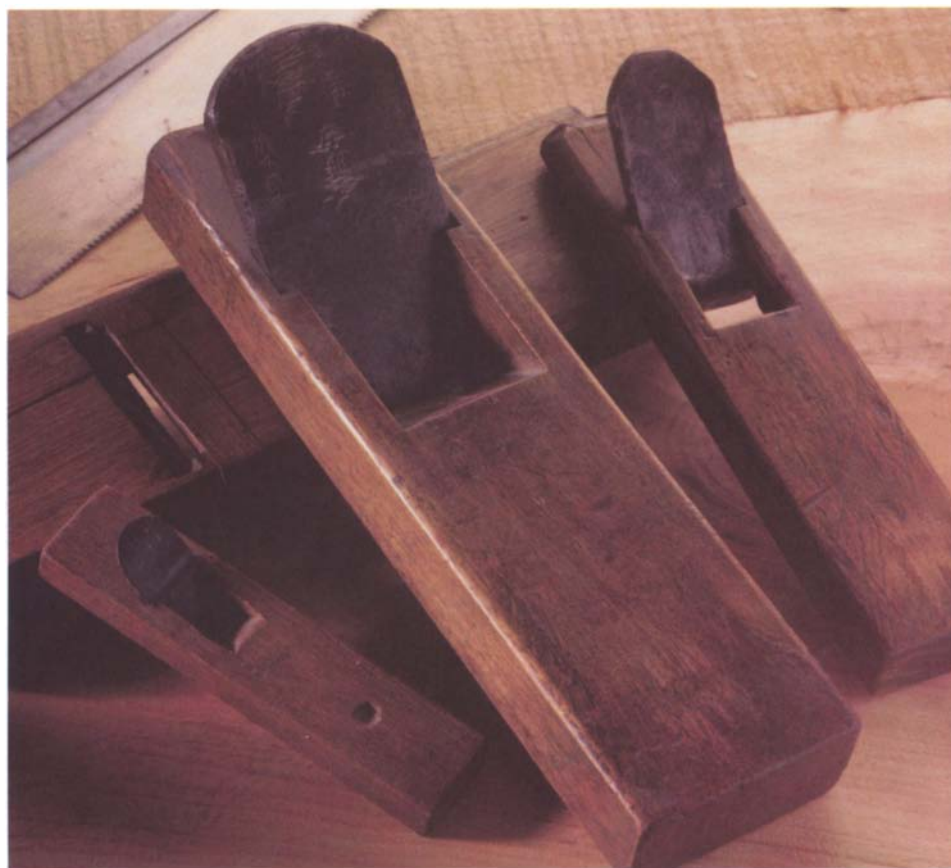
Oriental bench planes have thick irons and white-oak bodies. Notice the sliding dovetailed "key" to tighten the throat on the plane shown upside-down.
