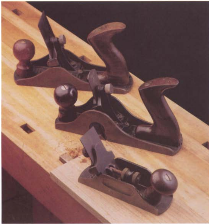
Similar to the bench planes they resemble, scraper planes have flat soles and strong handles. Shown here are three rare Stanley designs: from the top, a #87, a #85 with tilting handles, and a #212 that is used one-handed.
