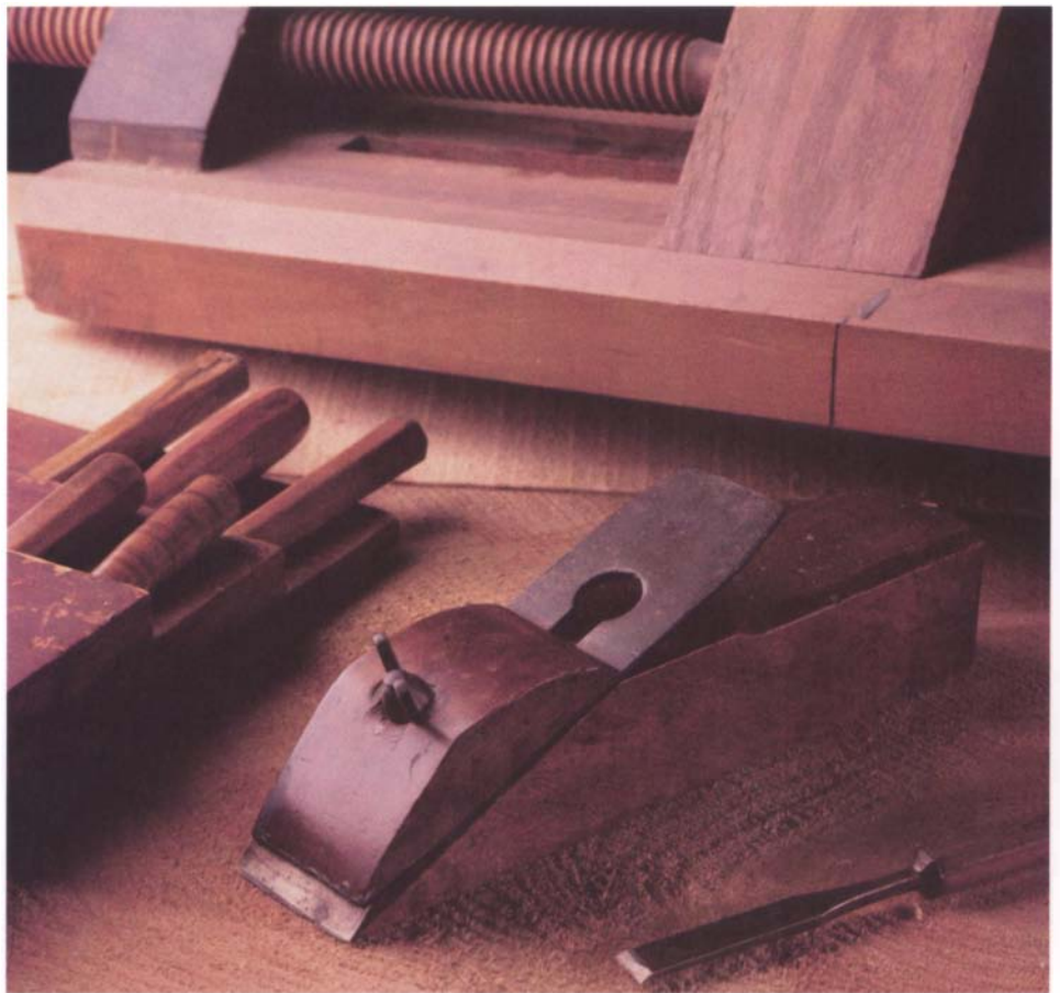
With the cutting edge right at the toe, this craftsman-made wooden chisel plane is ideal for working into tight corners or into areas inaccessible with other planes.
