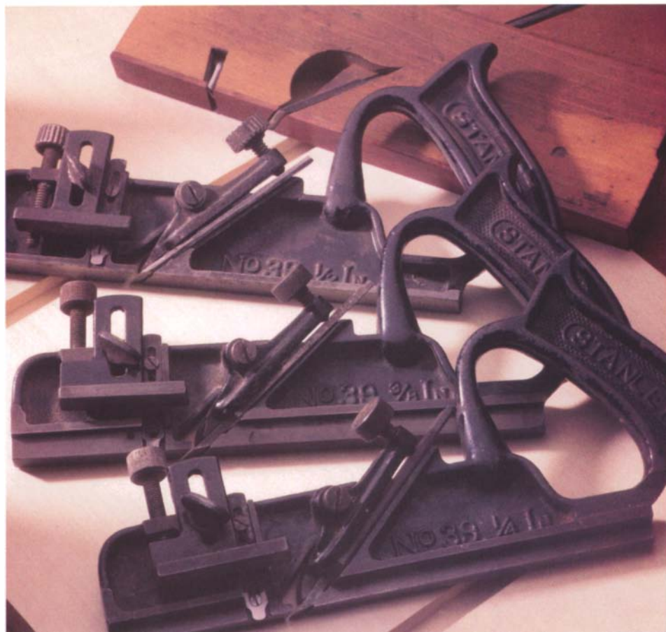
Stanley made a series of dado planes, with skewed irons, depth stops, adjustable nickers, and sole widths from \frac{1}{4} in. to 1 in. (#39 \frac{1}{4} , #39 \frac{3}{8} , and so on). The simple wooden rabbet plane in the background has a nicker iron wedged ahead of the main iron.
