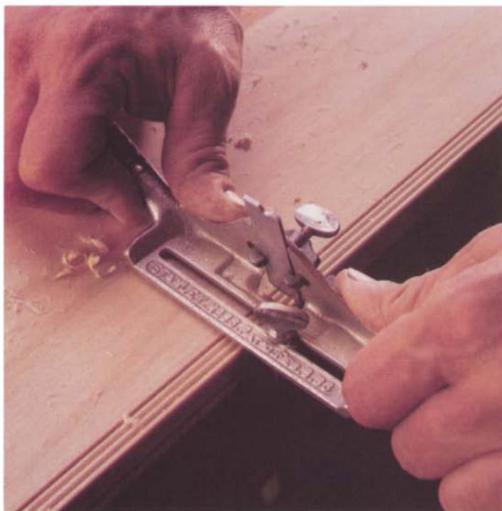
A Stanley #66 Universal beader is a good general-purpose holder for scratch tools. With different-shaped cutters and fences it can cut a wide variety of molding profiles, such as the triple reed shown here.
