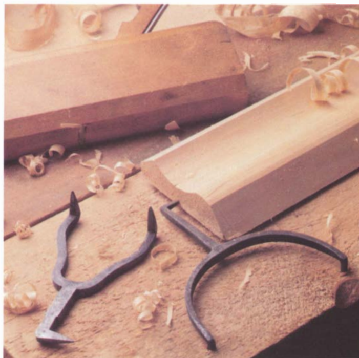
Forged-iron bench dogs can turn a plank into a quick planing bench.
