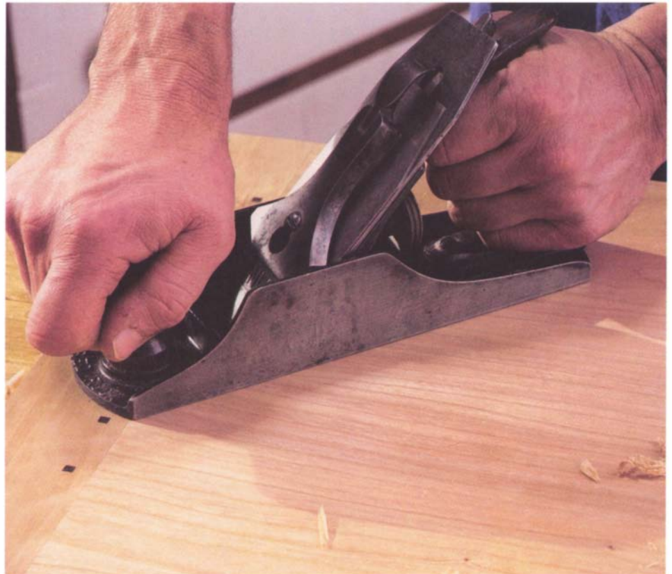
Smoothing a table with breadboard (or batten) ends poses a challenge. Plane up to the end, increasing the skew in the direction of the grain of the batten as you approach it. Just past the joint line, swivel the plane and finish the stroke along the batten.
