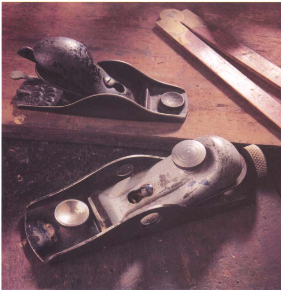
Schoolboy planes were made to be nearly indestructible, either with thick castings or made from pressed steel or malleable cast iron.
