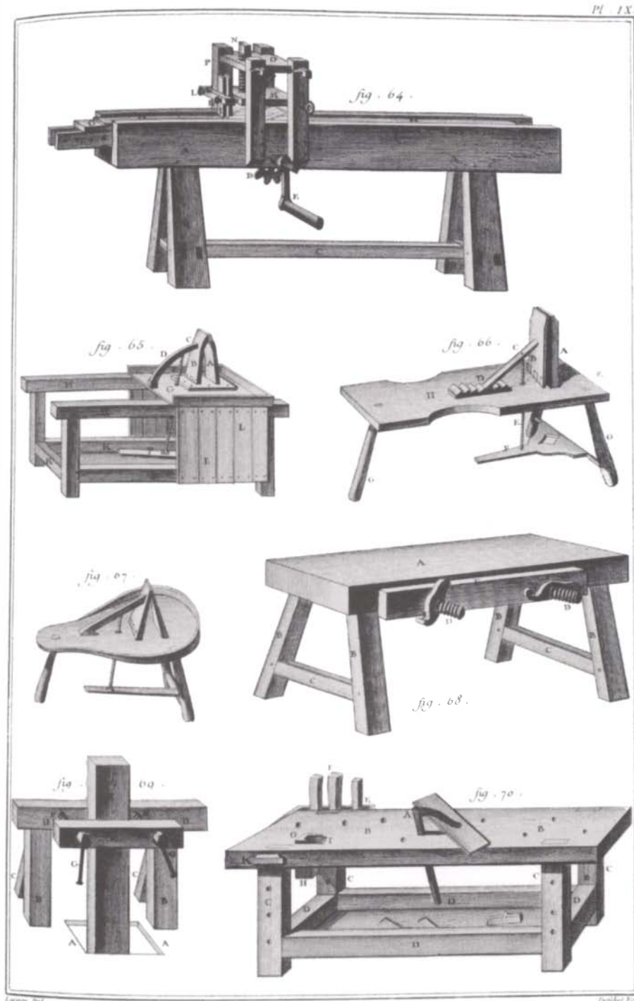
The simplest bench is part sawhorse, part flat benchtop. Adding a bench stop and an L-shaped holdfast greatly increases its versatility. (From Diderot's Encyclopédie .)
