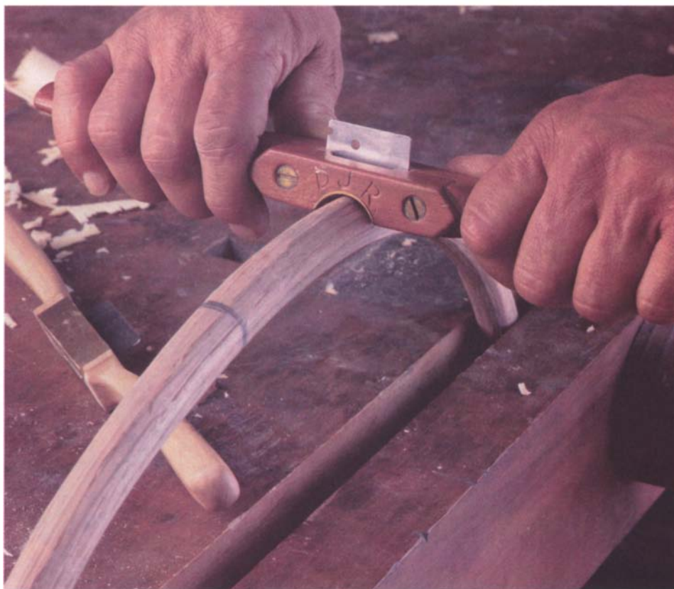
A chair devil will scrape complex shapes, such as the continuous back rail on this Windsor chair, a task nearly impossible with other planes. The tool on the bench is a flat-soled scraper.
