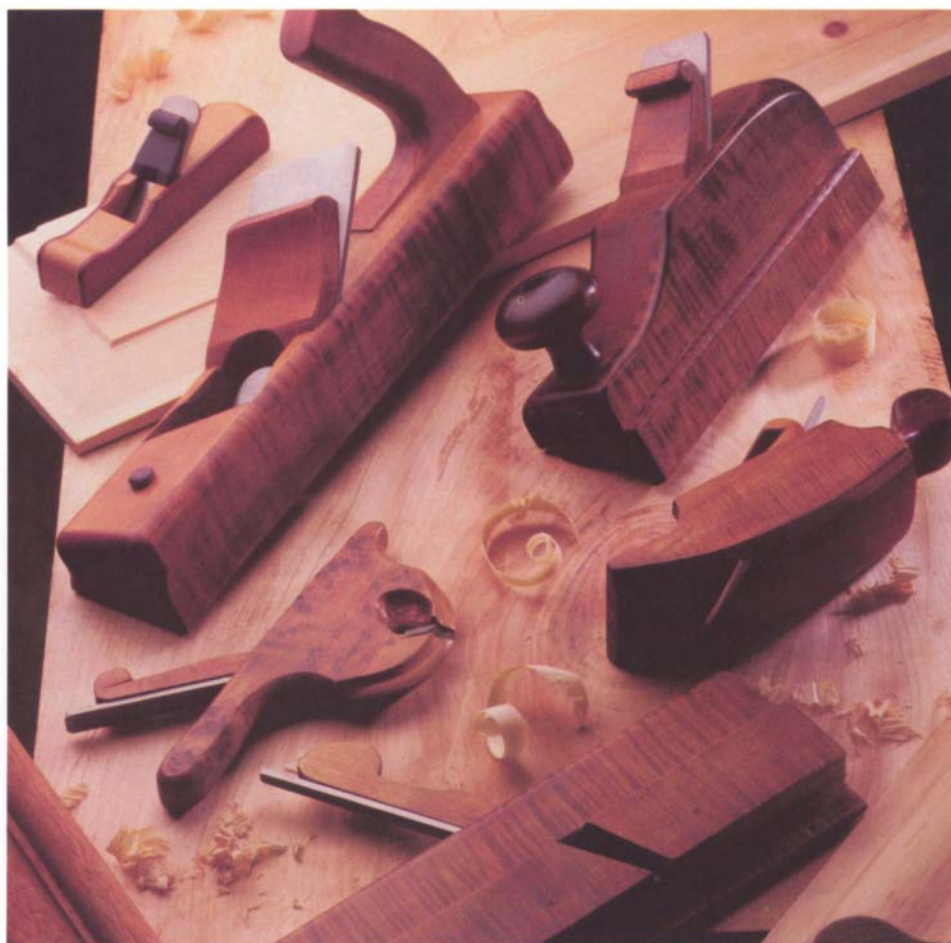
Leon Robbins makes traditional wooden planes. Shown here (clockwise from top left) are a miniature bench plane, a panel-raising plane, an unusual molding plane, a compass hollowing plane, a rabbet plane, and a coachmaker's plane.
