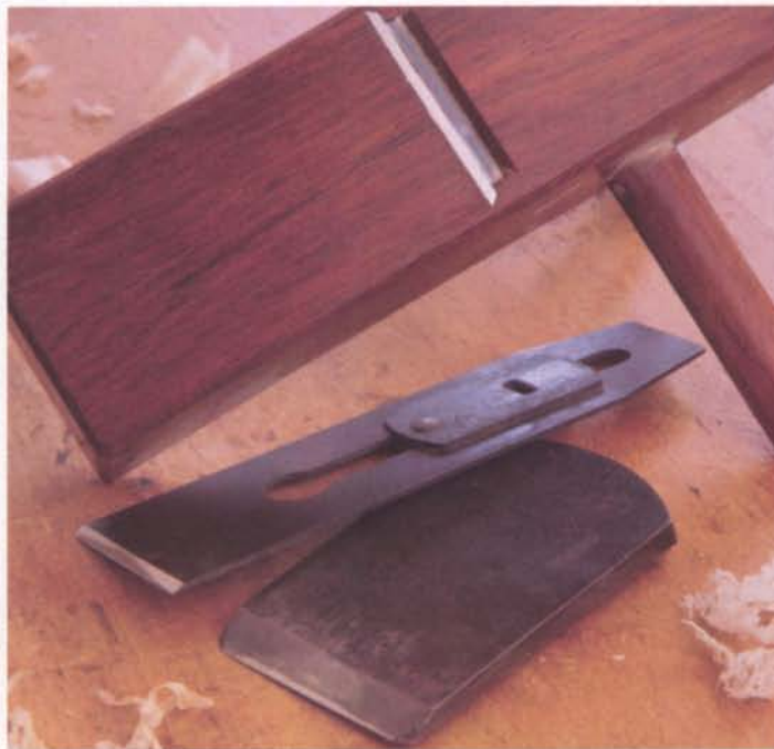
An Eastern plane iron (foreground) is considerably thicker than a standard Stanley bench-plane iron.
