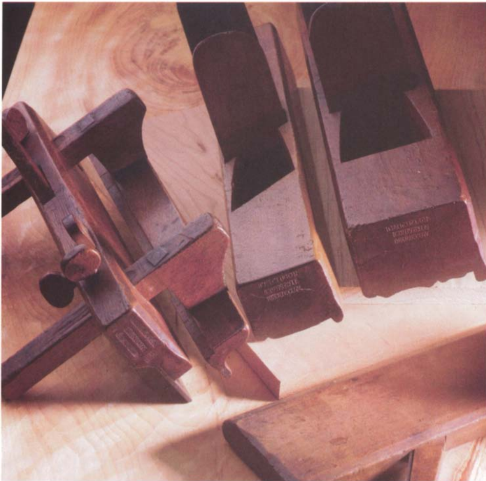
Early wooden-plane makers boldly stamped their names and towns into the toe of their planes. Shown here (from left) are a Nicholson plow plane with a fence riveted to the arms, a Chelor panel raiser, a Nicholson crown molder, and (in the foreground) a simple round.
