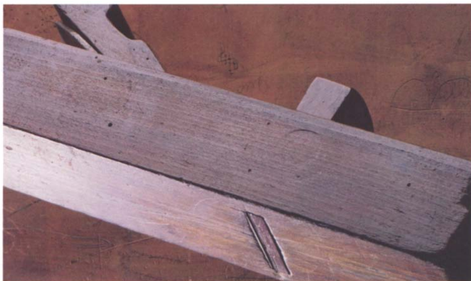
An ingenious way to tighten the throat on a wooden plane is with a wedge-shaped key let into the body, as on this English miter plane. Anytime the sole is jointed flat, driving the key in tightens the throat slightly.
