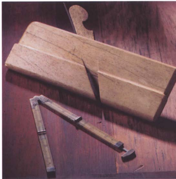
This unusual whalebone molding plane (a round) was possibly made aboard a whaling ship during the 18th or early 19th century.
