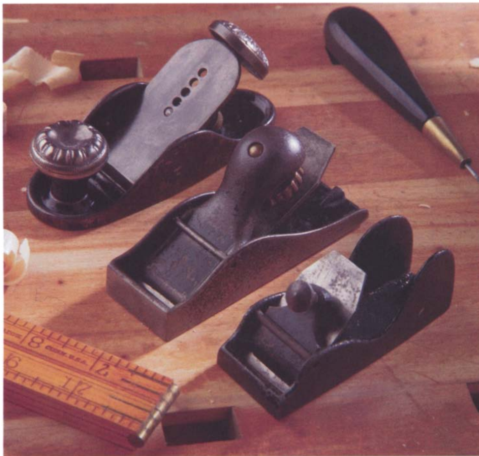
Block planes are useful for smoothing small surfaces and working in tight places. Shown here (from top) are a Leonard Bailey Victor #12½ with a decorative front and depth-adjusting knob and two English planes by Marples.
