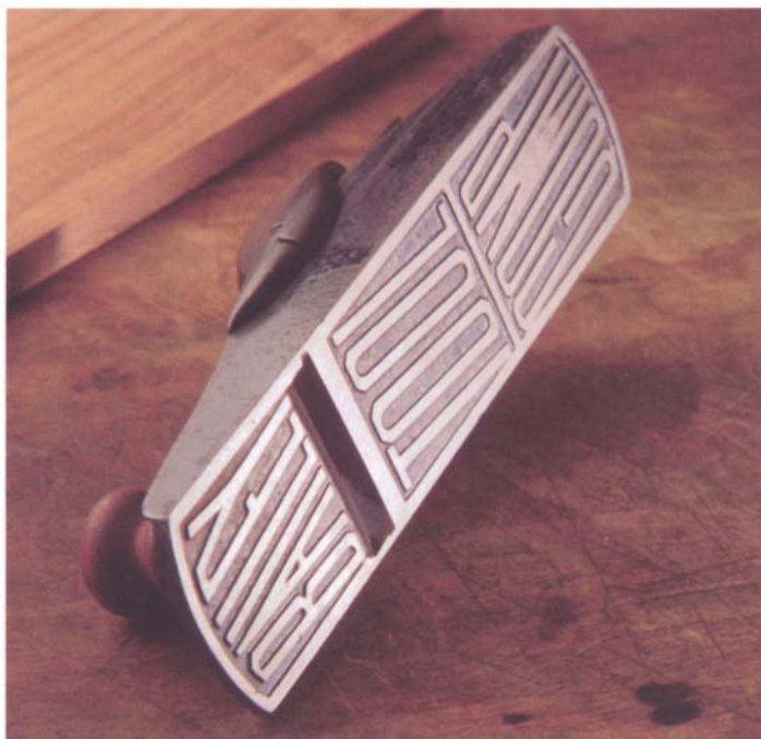
Corrugated soles could serve as advertising, too, as on this mid-1870s plane by the Bailey Tool Company of Woonsocket, Rhode Island. This company was started by Selden Bailey, not the better-known Leonard Bailey.
