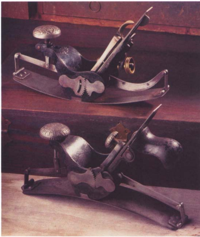
Two versions of Stanley's #113 compass plane. By turning the large knob, the flexible steel sole is pushed or pulled into a convex or concave circular radius.
