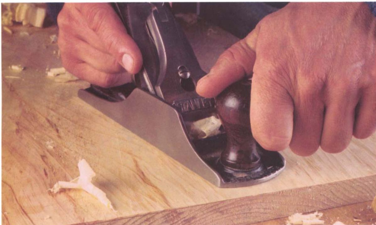
Working the surface on the diagonal, plane just to the gauge lines.
