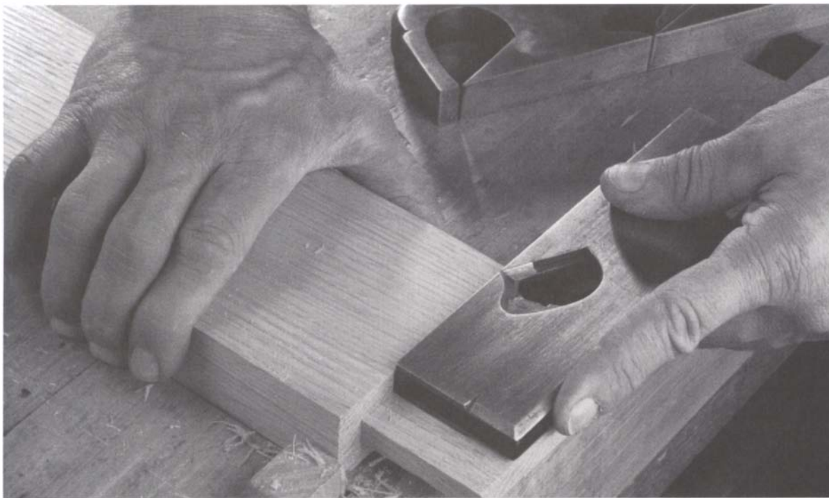
Use a shoulder plane, here a Spiers plane with rosewood infill, to adjust and true a tenon's shoulder.
