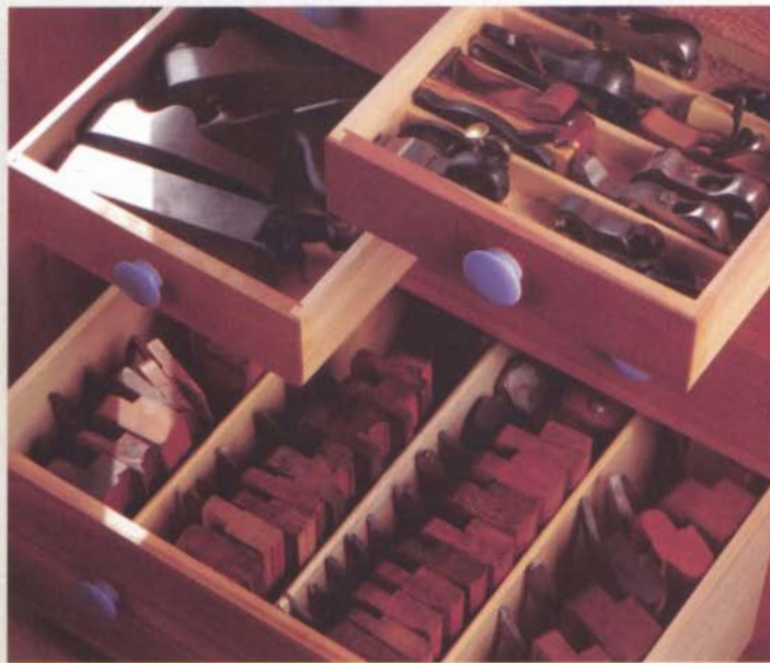
Drawers are an alternative for dust-free and efficient storage. They need to be designed to take a lot of weight and to fit planes of various dimensions.
