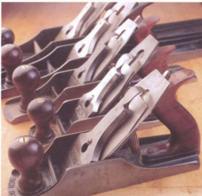
Bed Rock planes were made in a range of sizes from #602 to #608, with flat or corrugated soles.
