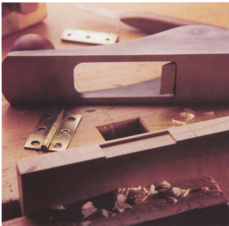
This butt mortise plane by C. M. Rumbold Co. has an unusually wide throat, so the user can see how the plane is cutting as it levels the bottom of hinge mortises or similar recesses.
