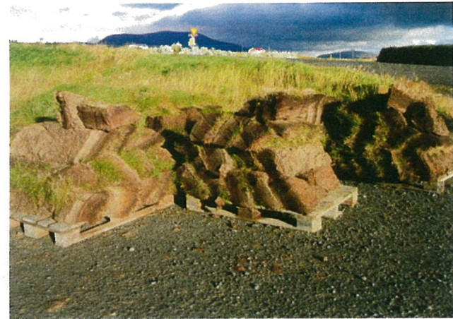
Here you see turf building materials, specifically clamped blocks that have finished drying and are stacked on pallets for transport.
