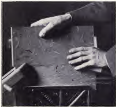
Fig. 261. Rubbing a Glued Joint.
