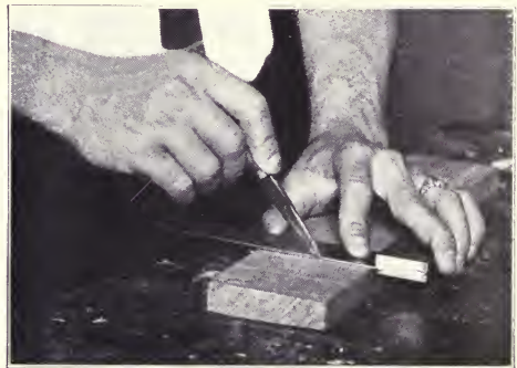
Fig. 204. Scribing with Knife by Try-Square.
