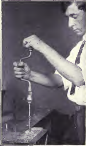
Fig. 137. Using a Try-Square as a Guide in Boring.
