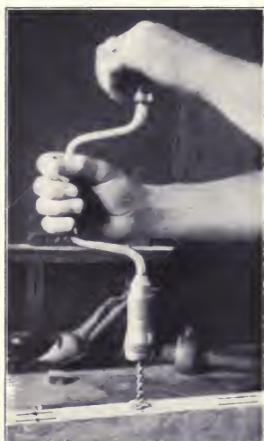
Fig. 263. Boring for Dowels in an Edge-to-Edge Joint.
