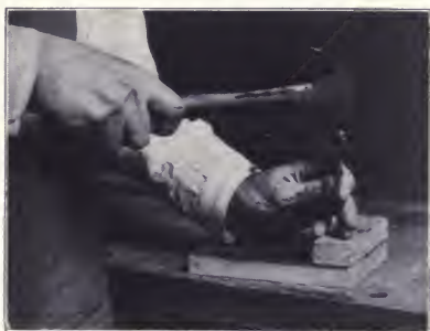
Fig. 165. Using a Nailset.
