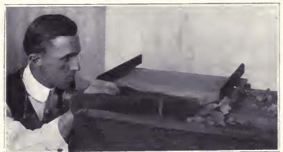
Fig. 206. Method of Using the Winding-Sticks.
