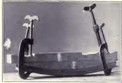
Fig. 299. Bending Boards into Shape after Boiling Them.
