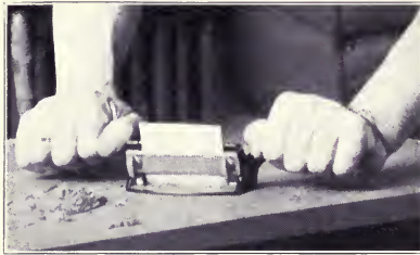
Fig. 151. Using a Veneer-Scraper.
