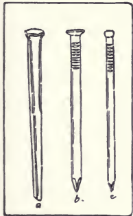
Fig. 226. a. Cut nail, common. b. Flat-head wire nail, No. 1, common. c. Finishing nail, or brad.
