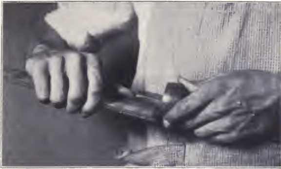
Fig. 213. Setting a Marking-Gage.
