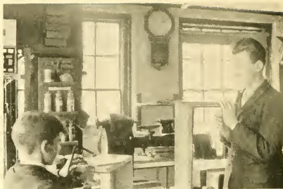
Boys using correctly the Supports for Coping Saw Work detailed in Plate 2.
