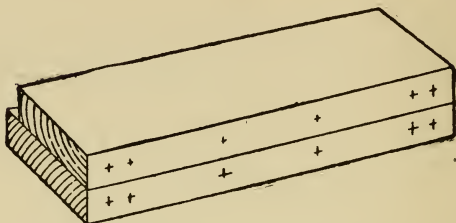
Fig. 200.—Marking and Gauging Boards for Dowelling.
