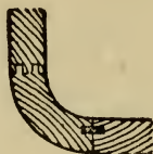
Fig. 110. Single Loose Tongue and Double- tongue Joint.
