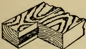
Fig. 101.—Joint with Single Dovetail Tongue and Groove.
