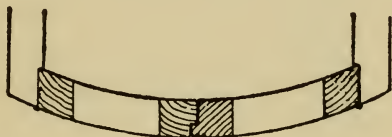
Fig. 262. Fig. 263.—Curved Cupboard Doors with Brass Astragal. Double-headed Rebated Joint.
