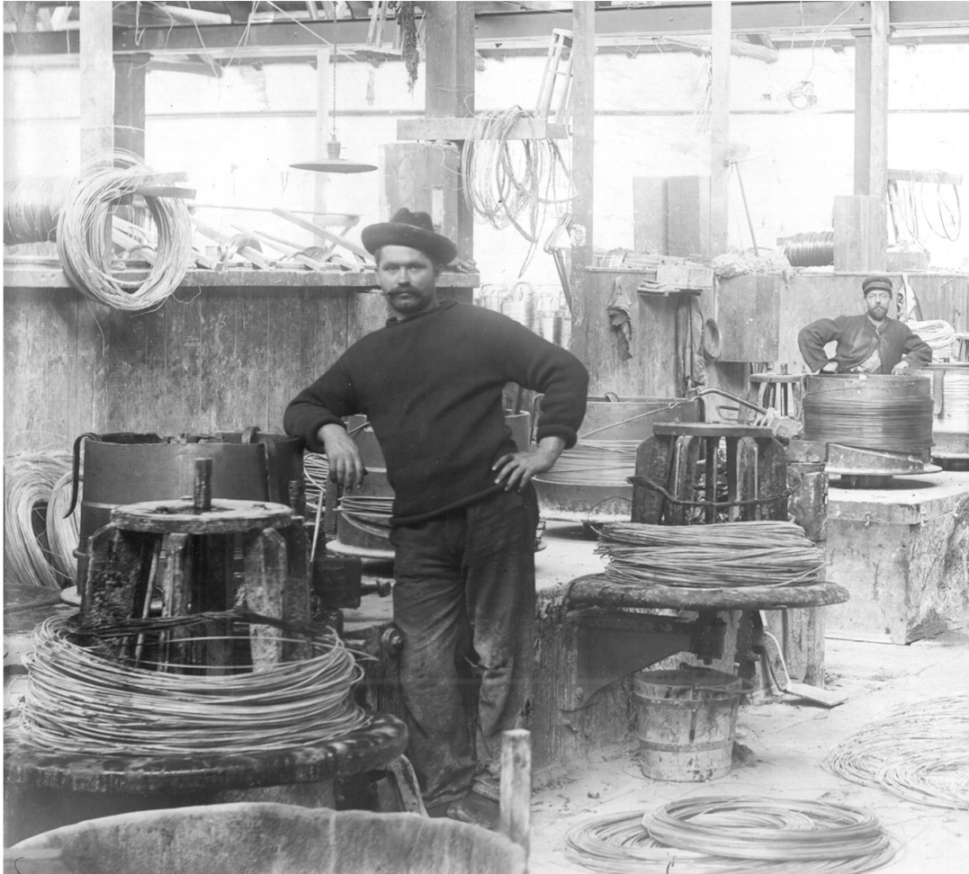
Fig. 1. Heavy equipment is necessary to draw the wire through the draw plate as seen in the first machinery at Traadværket around 1905 [Middelfart Museum].
