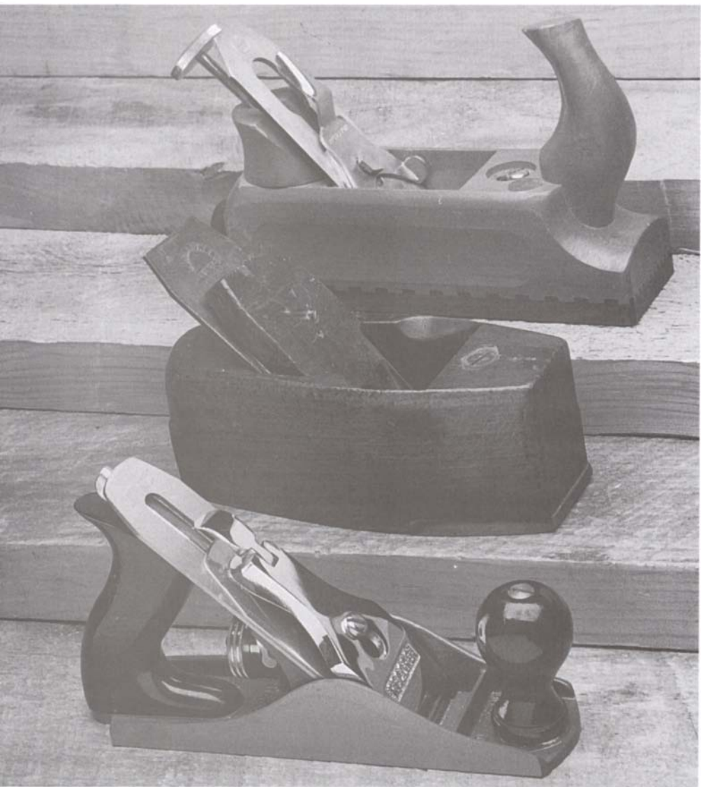
An adjustable mouth is desirable in any plane, but particularly in smoothing planes. The plane at top, of current German production, has a sliding insert in front of the mouth. The old smooth plane in the middle has an adjustable nosepiece much like modern block planes. The steel plane at bottom relies on a movable frog to open or close the mouth.
