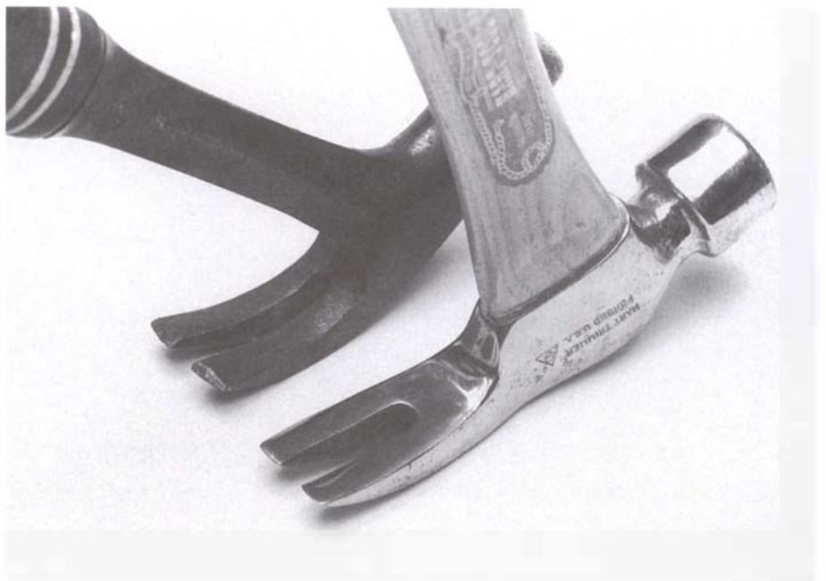
Hammer claws should be ground to smooth strong wedges, as shown on the hammer at front. The tips of the claws on the back hammer are much steeper than necessary. (Photos by Susan Kahn)
