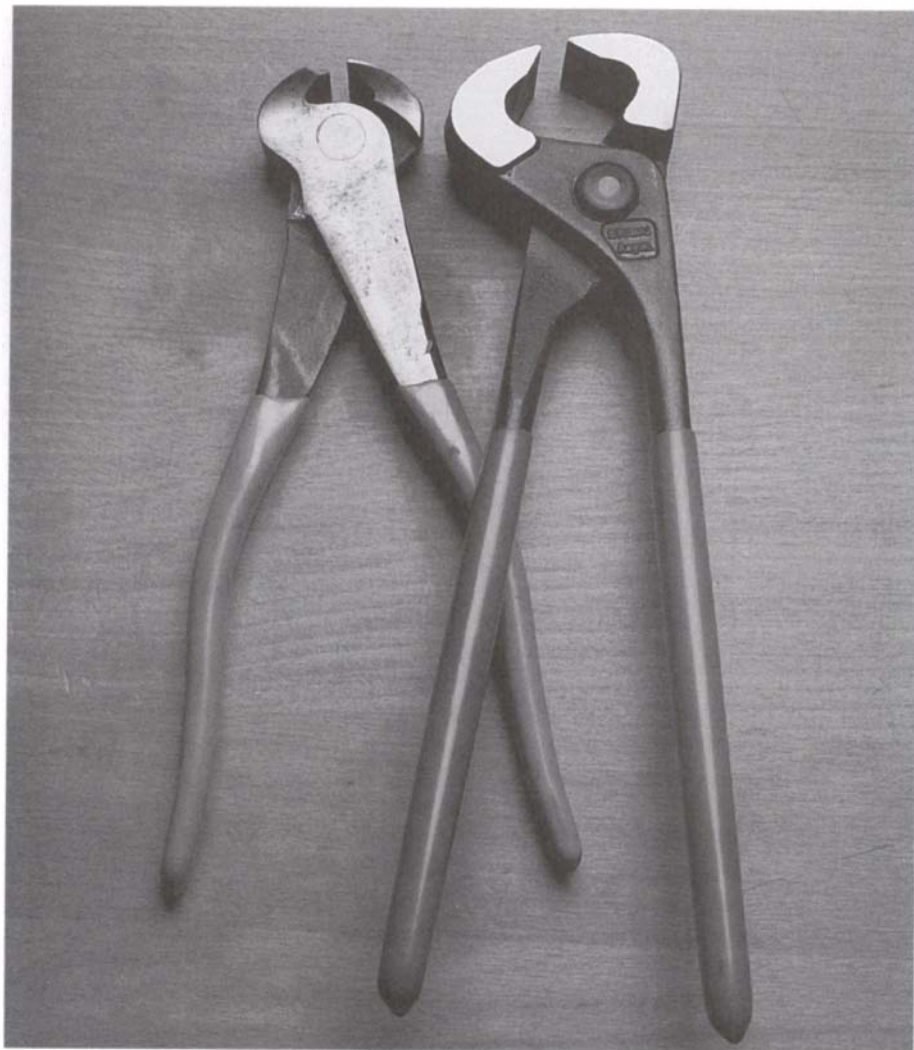
A nail puller (the longer-handled tool at right) can be used as an end cutter, although it is not as efficient because it is hinged well back from the jaw edges. However, an end cutter (at left) cannot be used as a nail puller because the jaws are too brittle (note the corner off one jaw).
