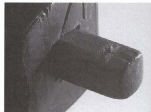
The stem of this old marking gauge has been scored by repeated filing of the marking pin.
