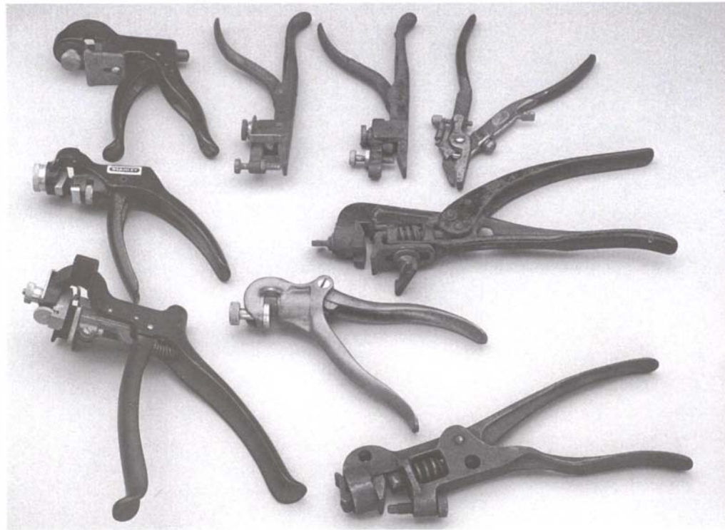
Like jointers, sawsets were (and still are) available in a wide range of styles, from the pistol-grip models at left to the plier styles at right.
