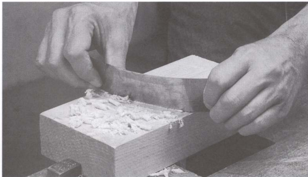
A well-sharpened cabinet scraper should make clean shavings, not dust. (Photo by Susan Kahn)
