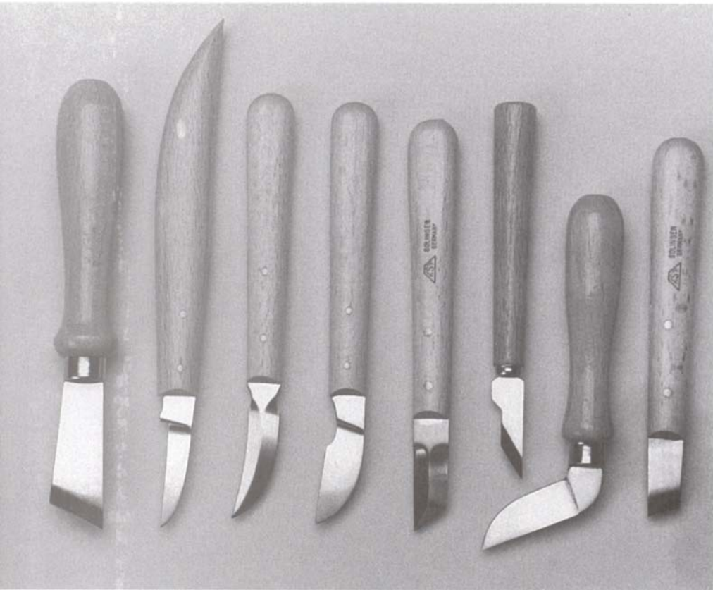
Chip knives are available in a wide range of styles. The knives second and third from left are more popular for carving in the round than for chip carving. (Photo by Susan Kahn)
