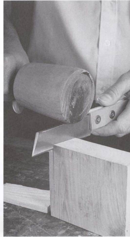
The thick blade and steep bevel angles of a hacking knife give it the necessary strength for rough work.
