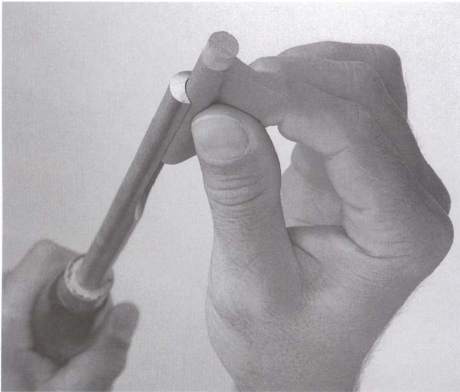
Using fine abrasive paper on a wooden dowel is one of the most effective ways to polish the flute of a gouge.
