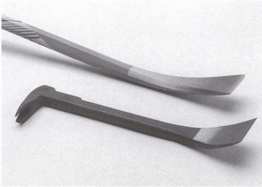
The prying tips of renovator's bars (back) and renovator's cat's paws (front) should be ground as thin as possible. (Photo by Susan Kahn)
