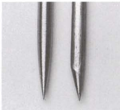
Concentric and eccentric trammel points. (Photo by Susan Kahn)
