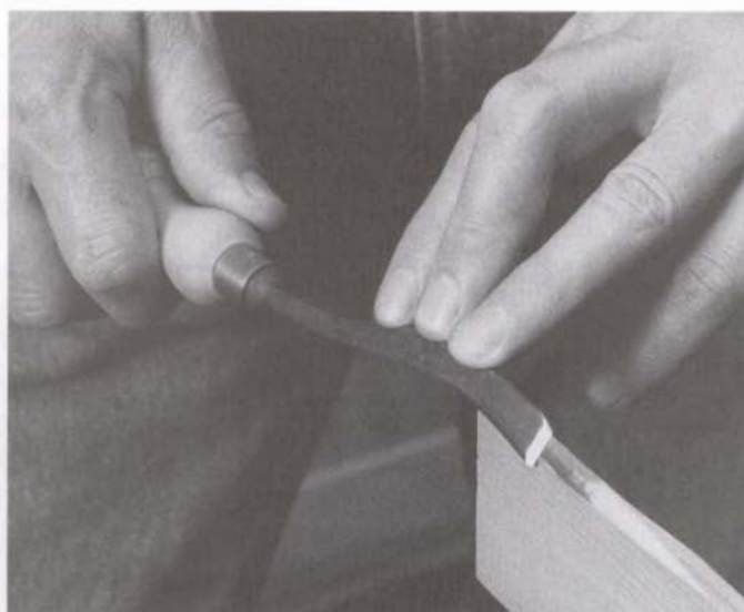
Hone the inside of a parting tool on a custom-made wooden form charged with honing compound. (Photos by Susan Kahn)
