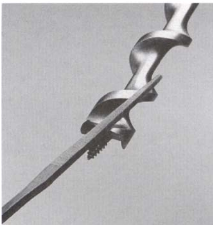
File the cutting lip of an auger bit with an upward stroke through the throat of the bit.
