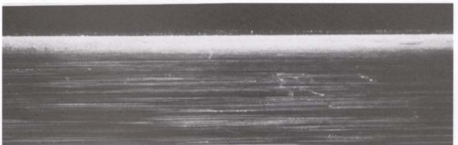
Three cabinet-scraper edges: at top, a sheared edge; in the middle, an edge after jointing with a file; at bottom, an edge (at greater magnification) showing the smoothing effect of stoning and burnishing. (Photos courtesy Canadian Conservation Institute)
