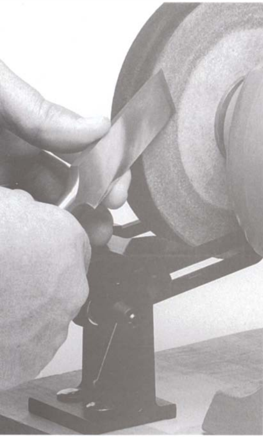
If you touch up chisels between sharpenings on a felt buffing wheel, use only the side of the wheel to minimize bevel rounding.
