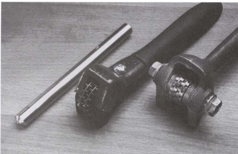
Tools for dressing grindstones include a diamond dresser (which can also be used for truing stones) and star-wheel dressers. The cutters of the star-wheel dresser at right have been worn through frequent use and are long overdue for replacement.
