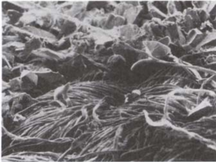
3M's diamond micro-abrasives on Mylar (top), paper (middle) and cloth backing (above). (Photos courtesy 3M)
