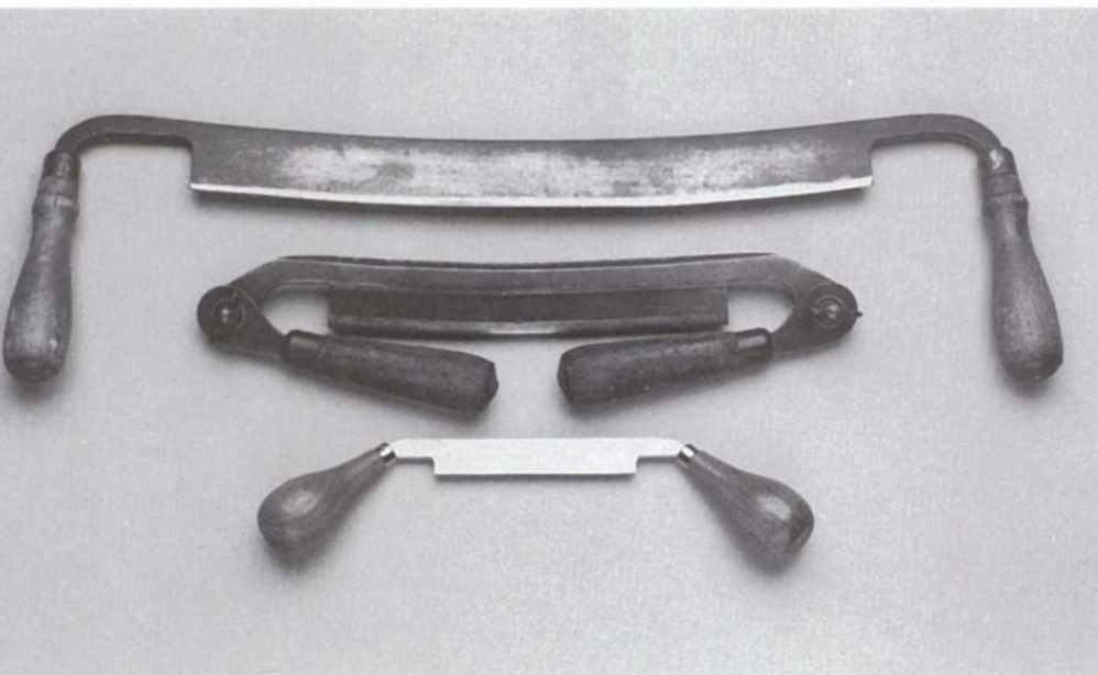
From top to bottom, a long drawknife for bark peeling, a classic carpenter's drawknife with folding handles to act as blade guards and a dainty carver's drawknife for fine work.
