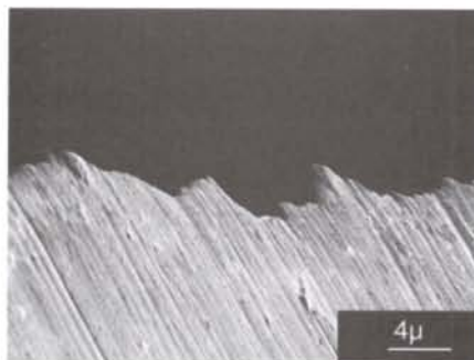
1. Bevel honed and stropped on green compound (face of chisel not lapped)
