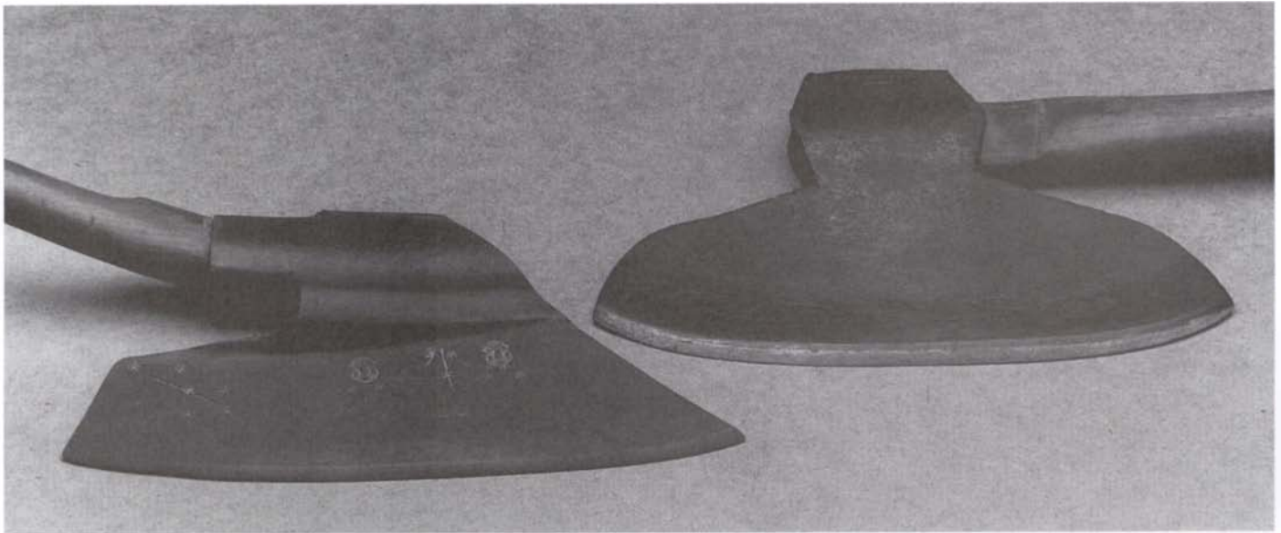
The European bearded ax (left) and the Canada-pattern broad ax (right) are the two most common styles of broad axes.
