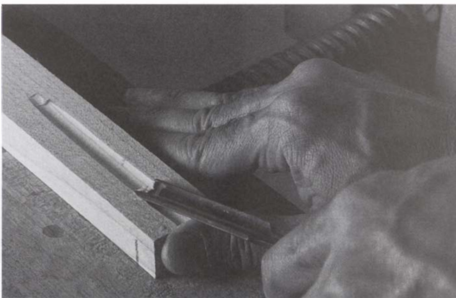
Cutting a groove in the face of a softwood block with a gouge produces a perfectly formed strop for honing the bevel of the same gouge. (Photo by Susan Kahn)
