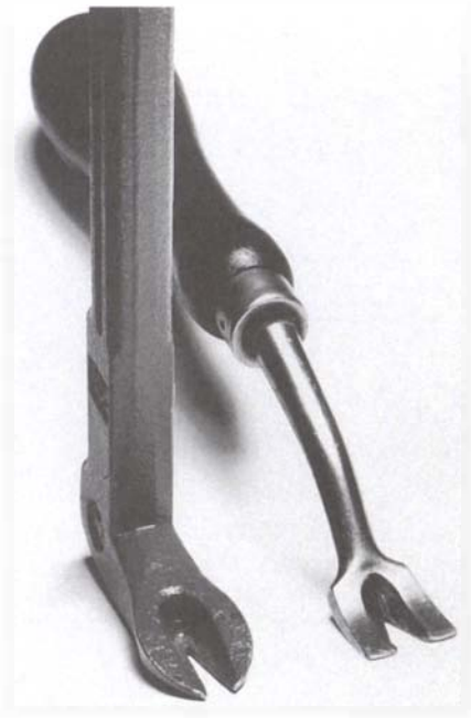
The claws of a Japanese cat's paw (left) are quite different from those of a traditional Western tack lifter (right). The relief grinding in the nail slot, the pointed tips and the rounded bottom differentiate them.
