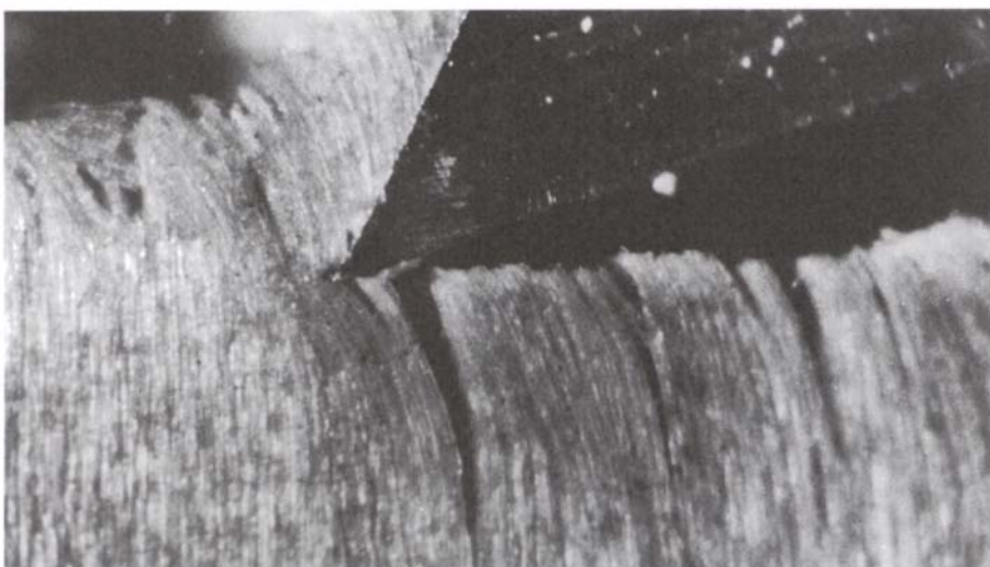
Top: Type I(a) failure in saturated eastern white pine; 40° rake angle; 0.010 in. chip thickness; 30x magnification.
