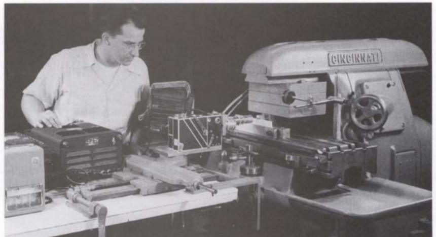
Dr. Norman Franz and his apparatus for recording the process of chip formation.
