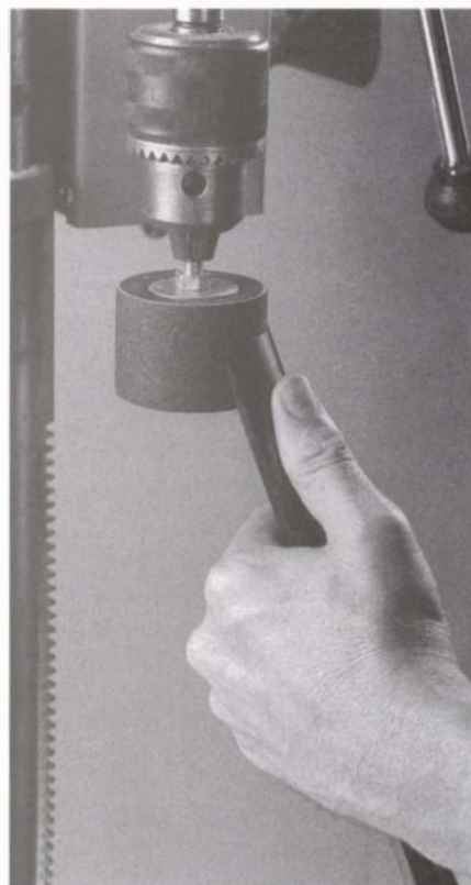
A sanding drum mounted in a drill press is a handy tool for sharpening large in-cannel gouges (left). The sanding drum can also be mounted in a flex shaft (above). (Photo at left by Susan Kahn)
