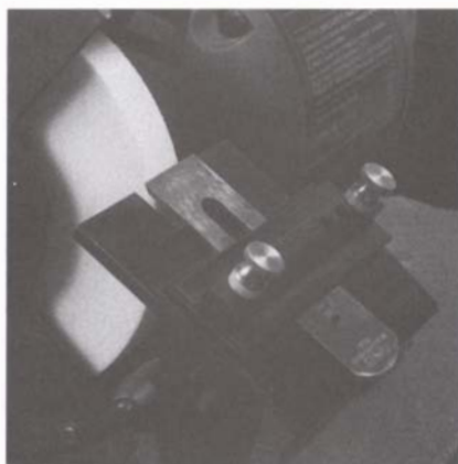
A jig that clamps the tool and can be slid across the tool rest is essential for accurate grinding. Shown here are a commercial jig (left) and a shopmade jig (right). (Photo at left by Susan Kahn)
