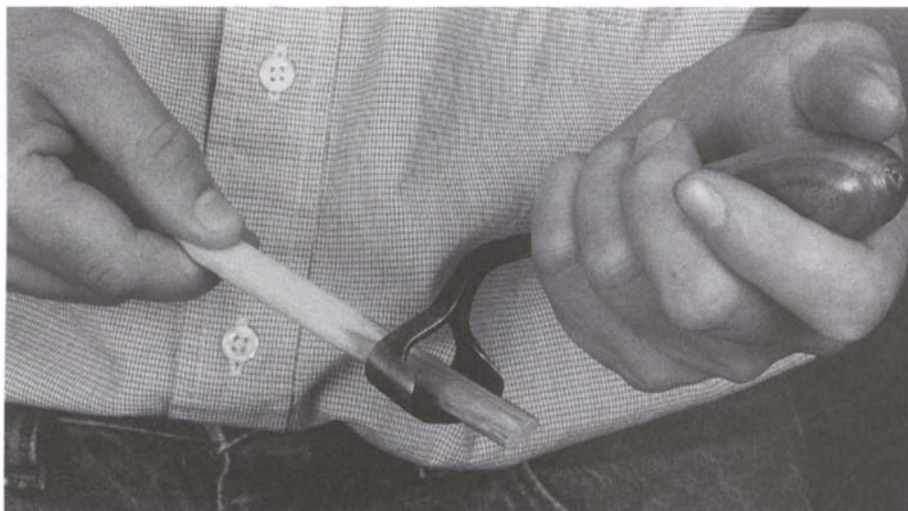
With the cutting edge of the tool facing away, use a chromium-oxide-charged wooden form to hone the inside of a scorp. Move the form much like a file, from the back inside of the scorp toward the edge. (Photo by Susan Kahn)
