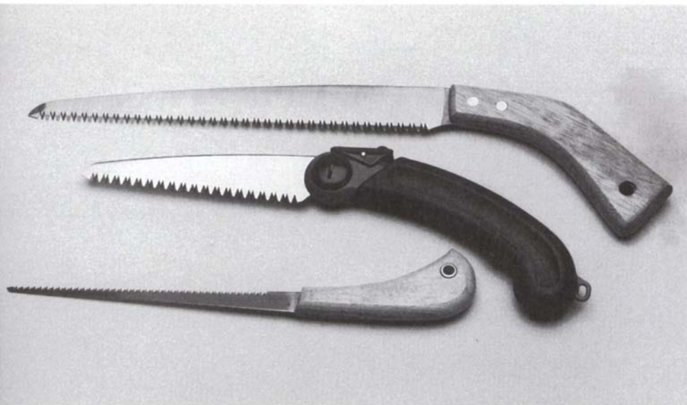
Two pruning saws and a keyhole saw. The saw at top, which has set teeth, is typical of Japanese pruning saws (though made in Taiwan). The middle saw, which has a tapered blade, is a top-of-the-line folding pruning saw made in Japan. The keyhole saw at bottom is just as effective in plasterboard as in wood. (Photo by Susan Kahn)
