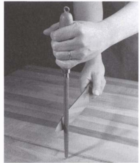
To use a knife steel, hold the steel vertically and take slicing cuts across it with the knife.
