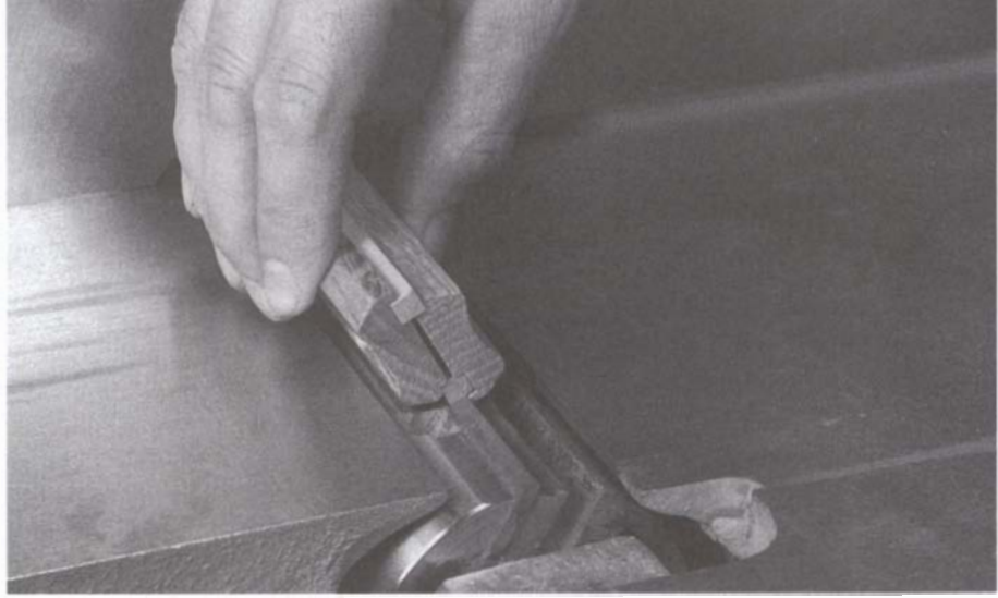
Commercial honing devices can be used to hone the bevel and deburr the knife edge. (Photo by Susan Kahn)
