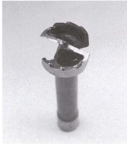
A sawtooth bit that has been jointed to make all teeth the same height.
