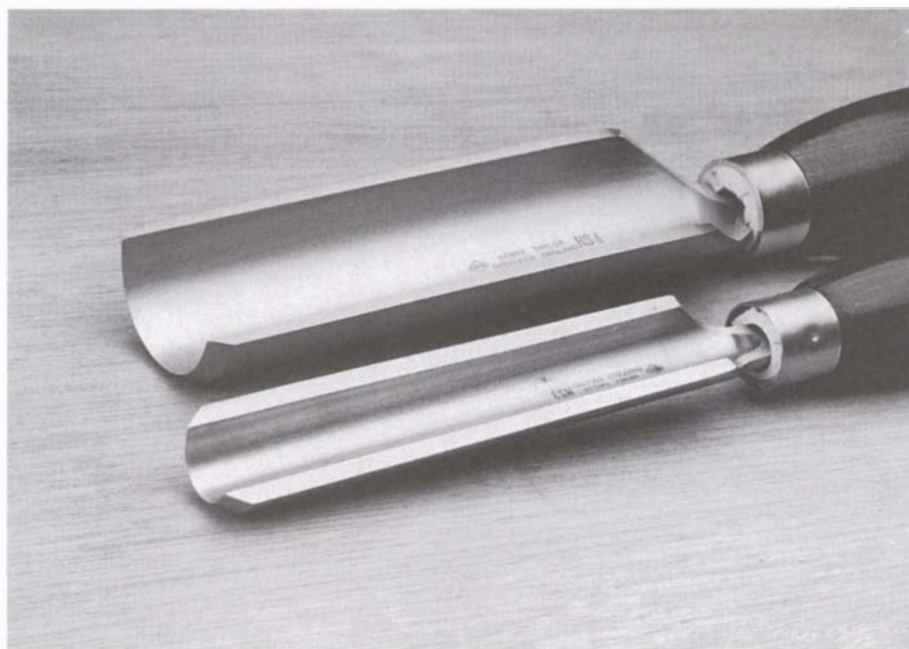
Roughing gouges, which are ground square across the tip, typically have a 45° bevel angle. These tools exemplify the design principle of form following function: The high wings clip fiber ends to prevent uncontrolled splintering as blanks are roughed down to size.
