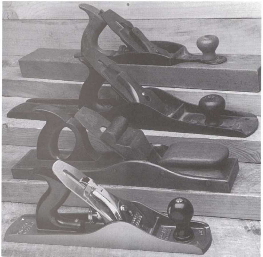
From top to bottom, a Bailey #30 jointer, a Stanley #7 jointer, a 16-in. craftsman-made panel plane and a Record #05 jack.
