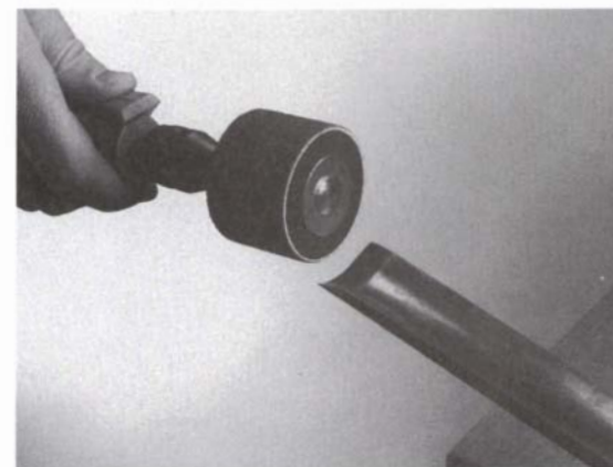
A sanding drum mounted in a drill press is a handy tool for sharpening large in-cannel gouges (left). The sanding drum can also be mounted in a flex shaft (above). (Photo at left by Susan Kahn)
