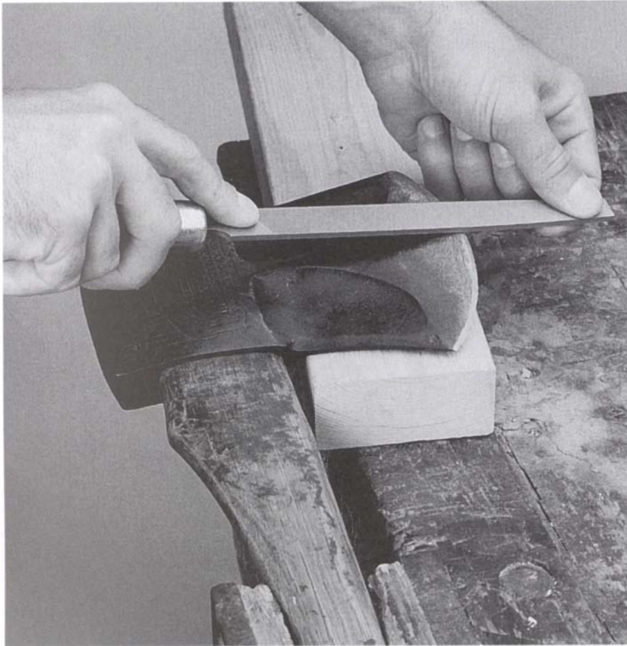
Using an 8-in. mill file, file the ax away from the edge.
