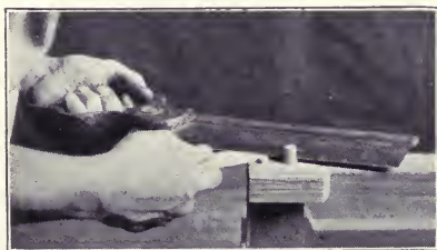
Fig. 139. Sawing off projecting end of dowel-pin.
