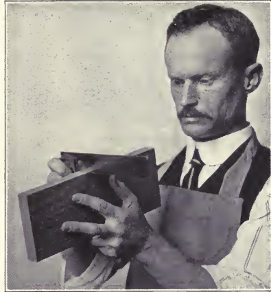
Fig. 24. Testing an edge for squareness.
