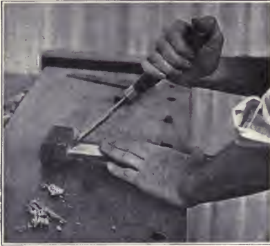
Fig. 41. Trimming a miter.
