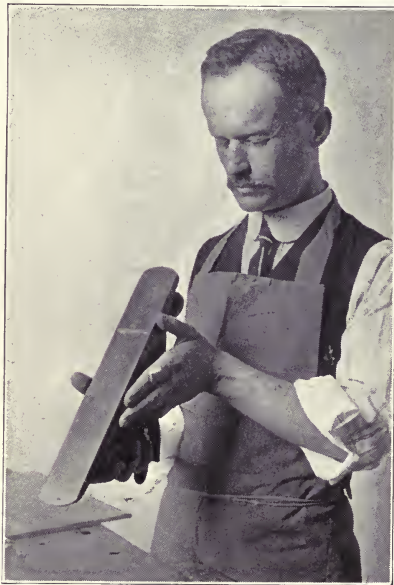
Fig. 21. Sighting along the sole of the plane to see that the cutter is properly adjusted.
