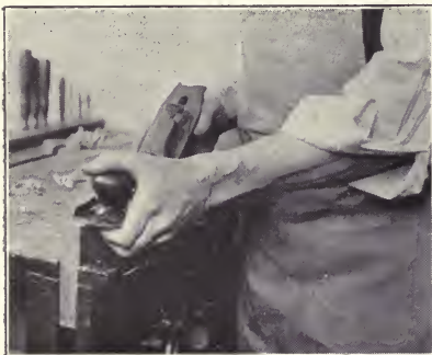
Fig. 25. Holding the plane so as to square up a beveled edge.
