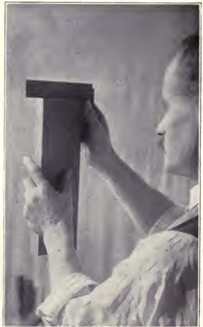
Fig. 27. Testing squareness of end.
