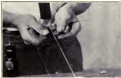
Fig. 86. Breaking the glass. (Step 3.)
