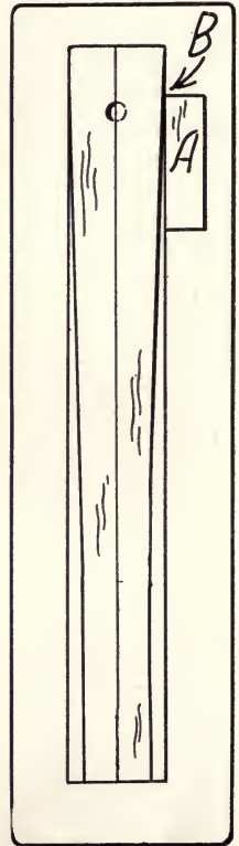
Fig. 162. Method of starting saw on a tapering cut.
