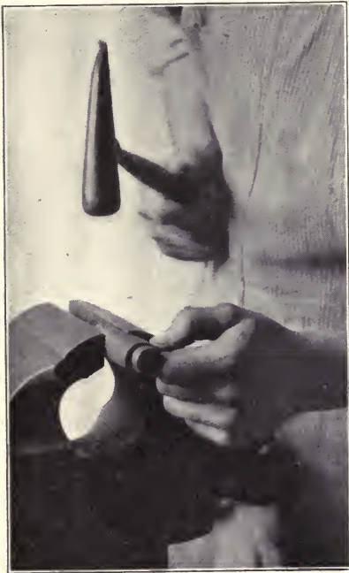
Fig. 108. Hammering a strip into a cylinder.
