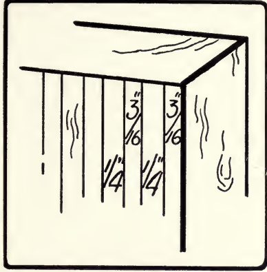
Fig. 28. Gaged lines on piece to be sawed into slats. The saw-kerfs are to be in the middle of the \frac{1}{4} " spaces.
