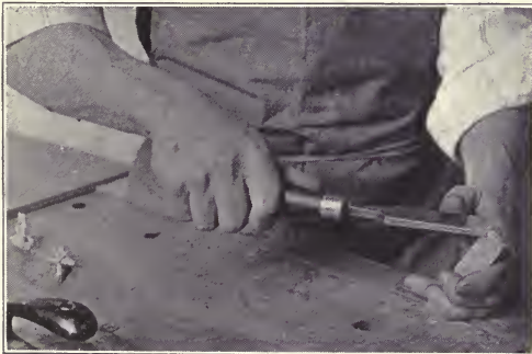
Fig. 33. Slicing off an arris with a chisel.
