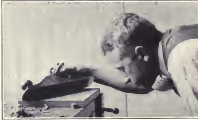
Fig. 34. Testing a planed surface for flatness by using the arris of the plane.
