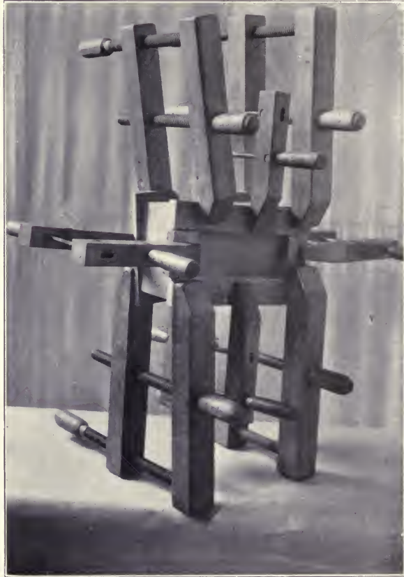
Fig. 192. Gluing the top on to the box.
