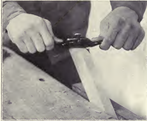
Fig. 57. Using the spokeshave.
