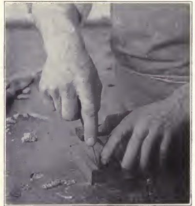
Fig. 35. Scoring with a knife along the try-square.
