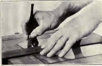
Fig. 84. Cutting glass. (Step 1.)
