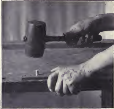
Fig. 132. Driving dowel thru dowel-plate.
