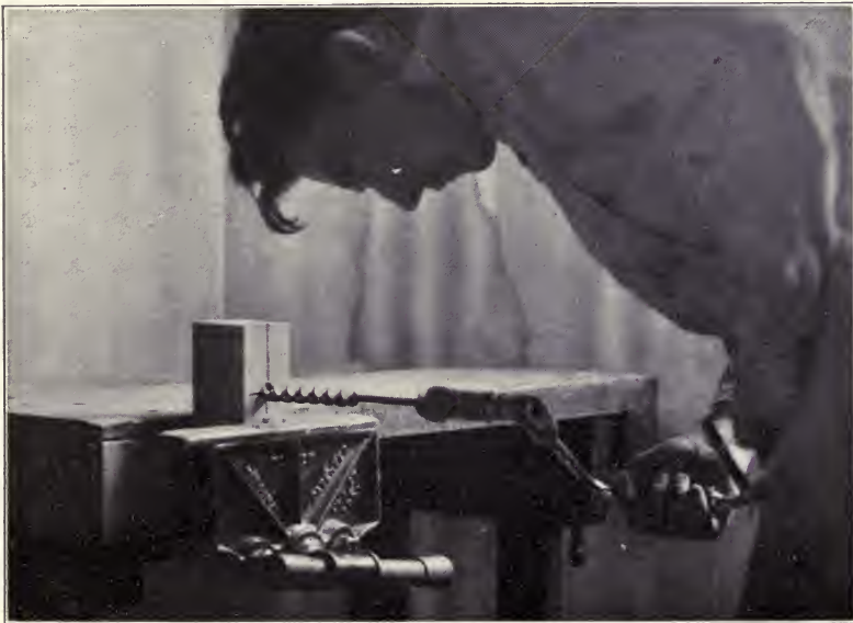
Fig. 156. Boring hole in head of mallet.
