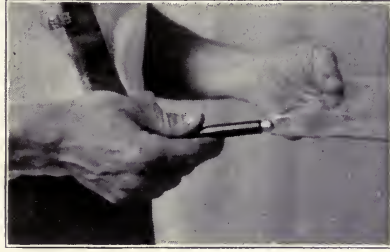
Fig. 85. Tapping under the scratch in the glass to start a crack. (Step 2.)
