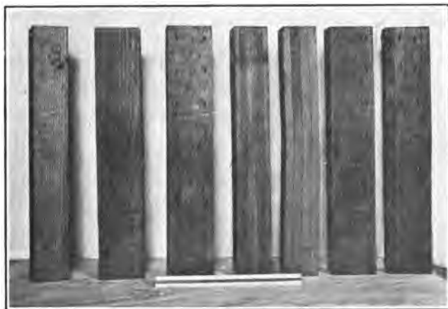
FIG. 64. TEST-COLUMNS AFTER FAILURE.
