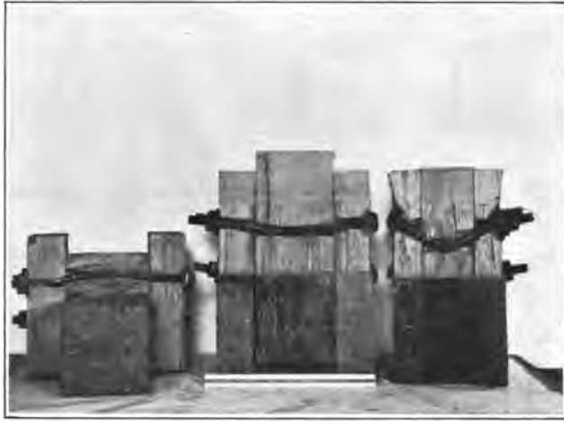
FIG. 35. PHOTOGRAPH OF JOINTS AFTER TESTING.
