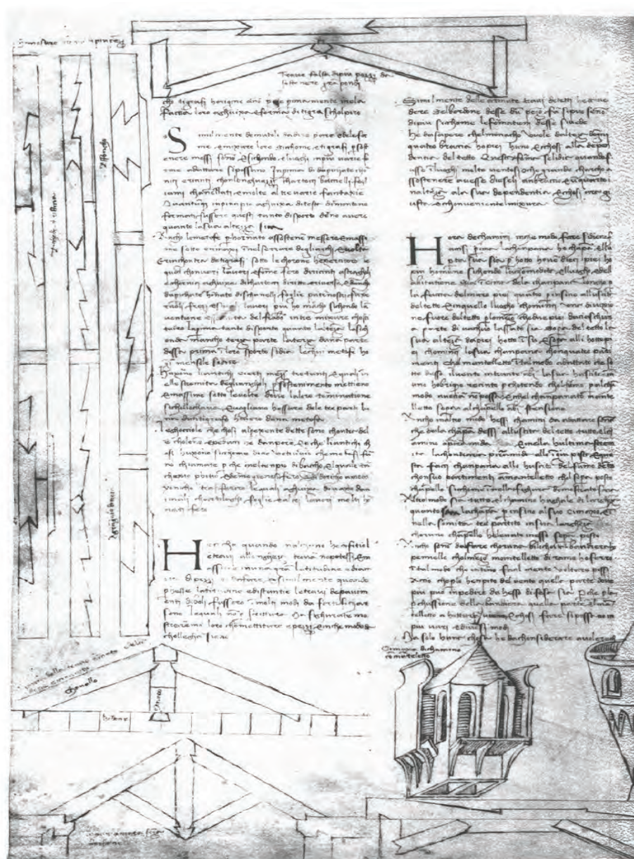
Fig. 11: Francesco di Giorgio Martini, various methods for increasing the length of horizontal beams (Martini [1470–1490] 1967, Tomo 1, p. 96).
