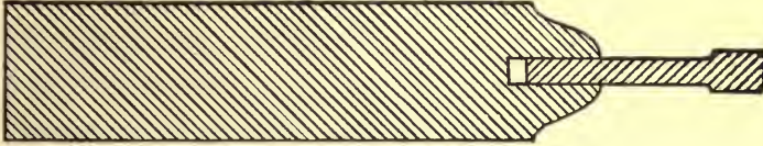
Fig. 53. Section of Solid Door.
