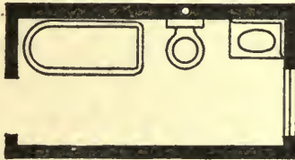
Fig. 6. Layout of a Very Small Bathroom.
